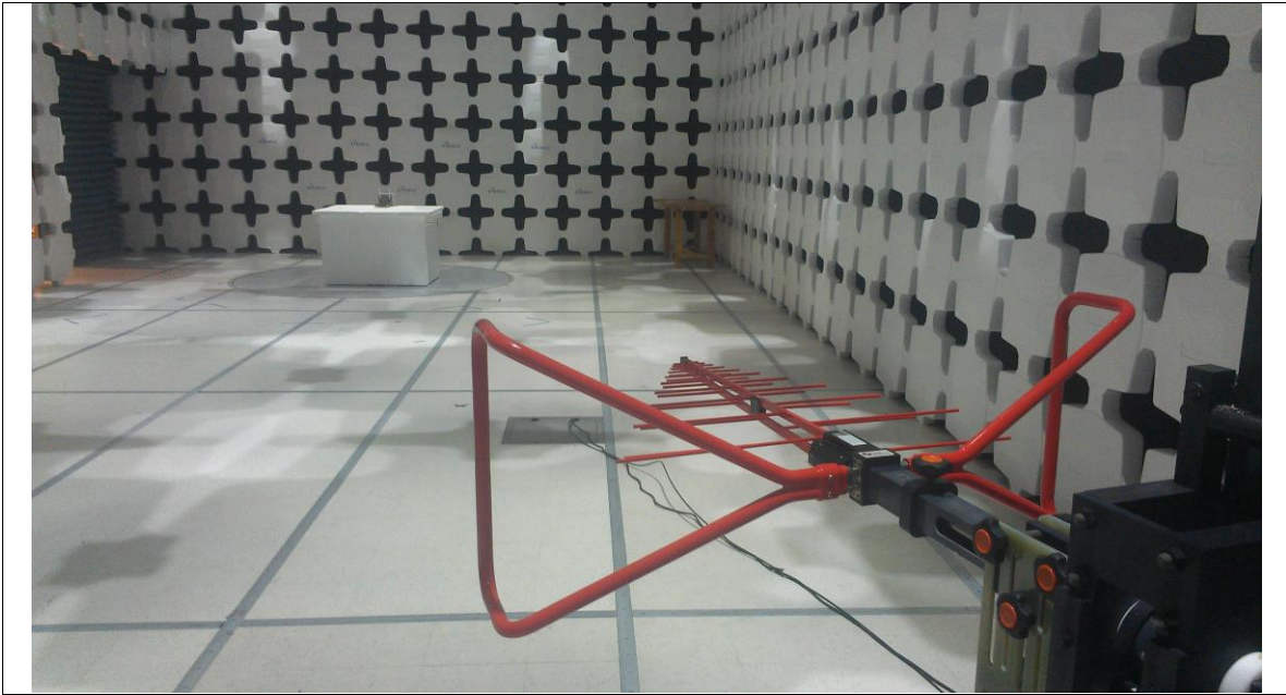
Radiated Emission Test Setup (below 1GHz) with Sleeve antenna: Sansei - Front View
