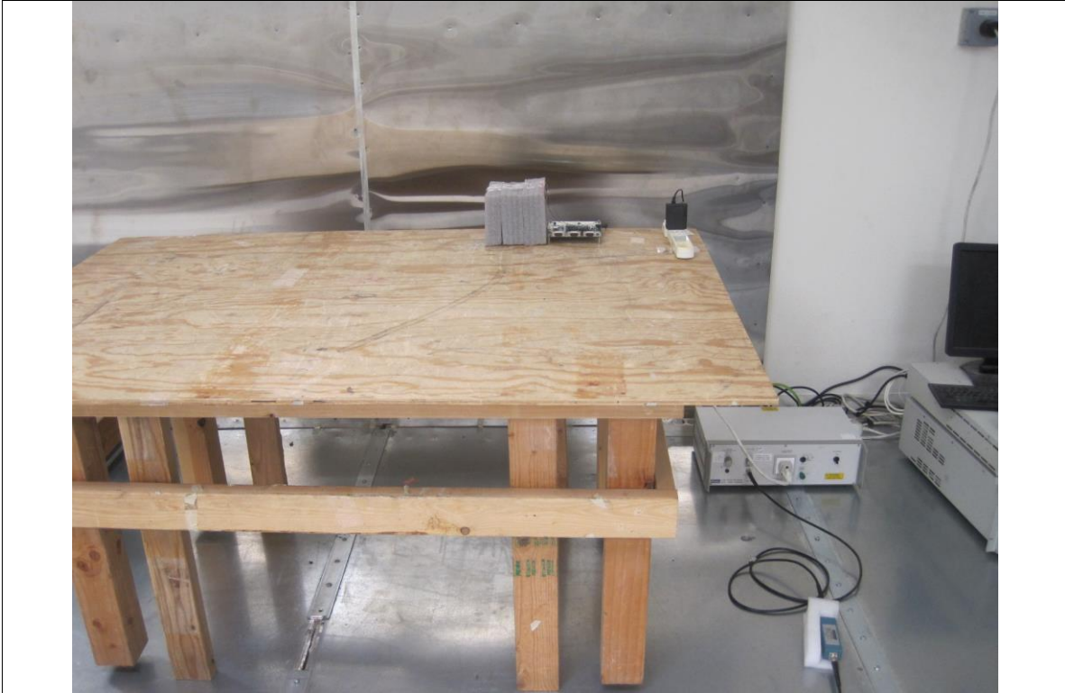
Conducted Emission Test Setup (below 1GHz) - Front View
