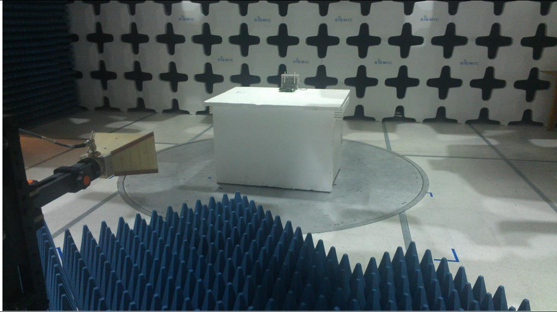
Radiated Emission Test Setup (above 1GHz) with Sleeve antenna: Sansei - Front View
