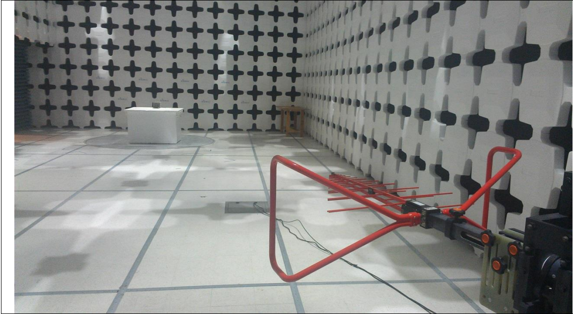
Radiated Emission Test Setup (below 1GHz) with Embedded antenna: Ethertronics - Front View
