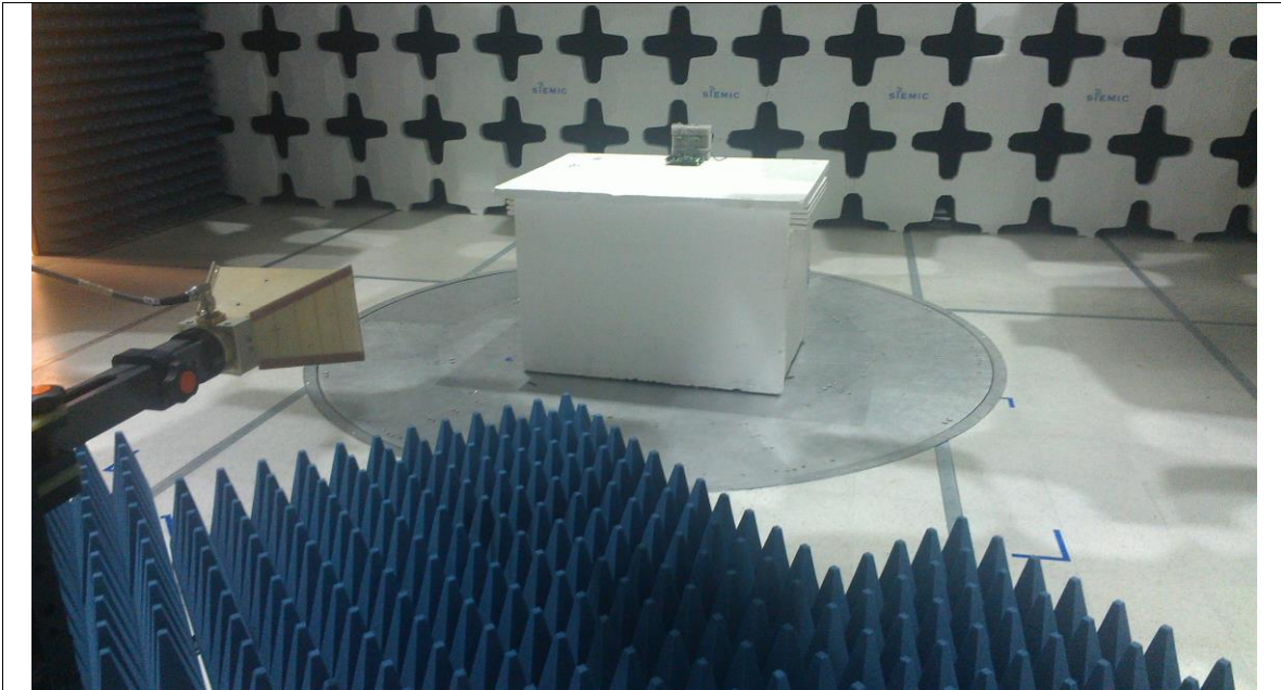
Radiated Emission Test Setup (above 1GHz) with Embedded antenna: Ethertronics - Front View
