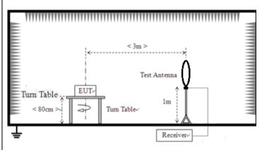
For radiated emissions from 30MHz to1GHz
