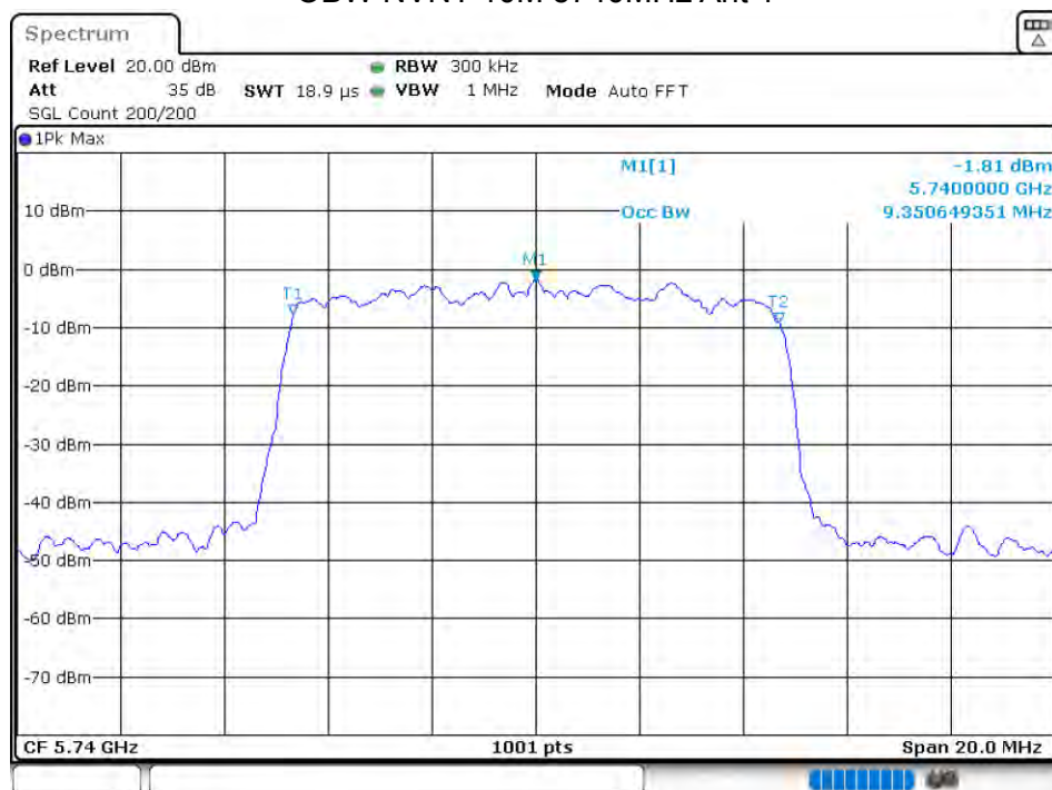
OBW NVNT 10M 5740MHz Ant 1
