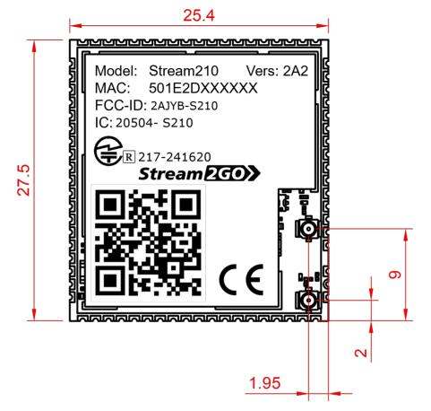
Each module is individually identifiable with a sticker or laser engraving method.
