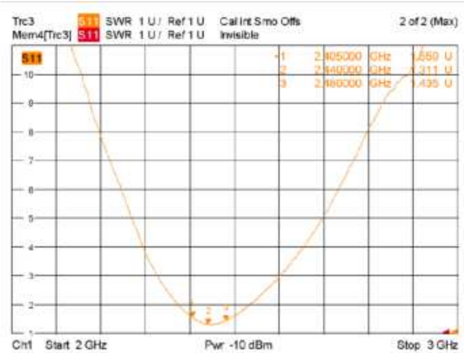
Figure 10: VSWR with Module Installed in the Upper Right Corner (Position #3) of the Evaluation Board
