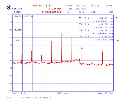
Plot # 17 : Spurious Emission Conducted at Antenna terminal, Low power setting Frequency: 896 MHz, Modulation: 2-Level 8kbps GMSK
