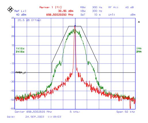
Plot # 7: Emission Mask J, , RF Output, High Power Setting Frequency: 901 MHz, Modulation: 2-Level 8kbps GMSK
