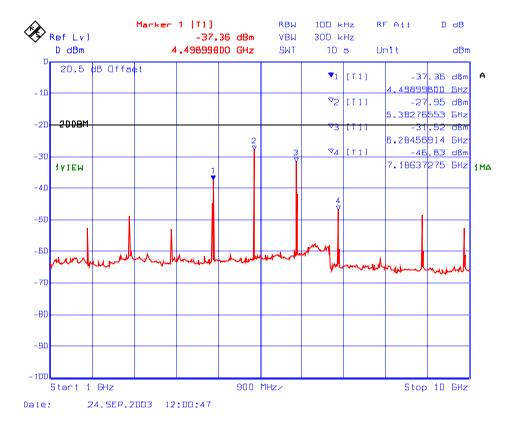
Plot # 15 : Spurious Emission Conducted at Antenna terminal, High power setting Frequency: 901 MHz, Modulation: 2-Level 8kbps GMSK
