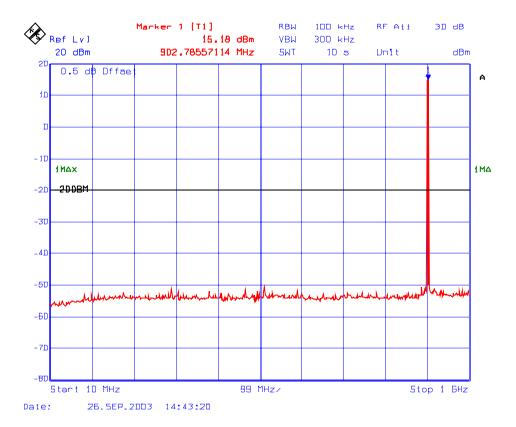
Plot # 22 : Spurious Emission Conducted at Antenna terminal, Low power setting Frequency: 901 MHz, Modulation: 2-Level 8kbps GMSK
