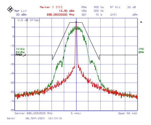
Plot # 9: Emission Mask J, , RF Output, Low Power Setting Frequency: 898.5 MHz, Modulation: 2-Level 8kbps GMSK
