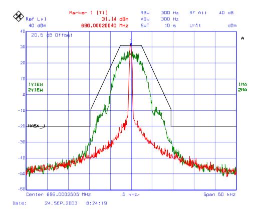
Plot # 6: Emission Mask J, , RF Output, High Power Setting
