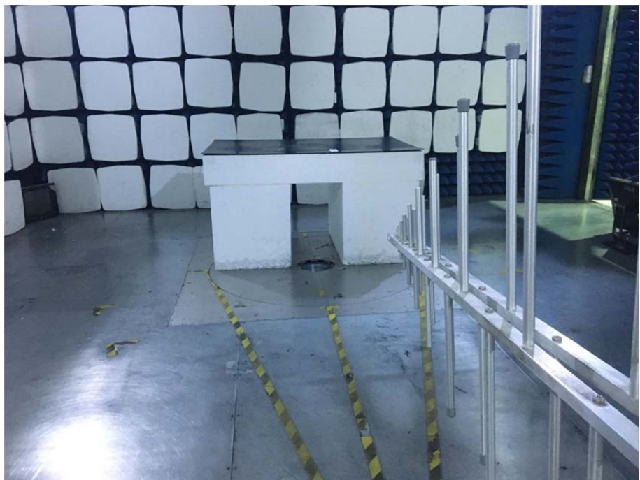
Radiation Emission Test Setup (30MHz to 1GHz)
