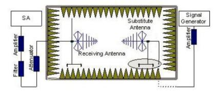
In the chamber, an substitution antenna for the frequency band of interest is placed at thereference point of the chamber. An RF Signal source for the frequency band of interest isconnected to the substitution antenna with a cable that has been constructed to not interfere with
