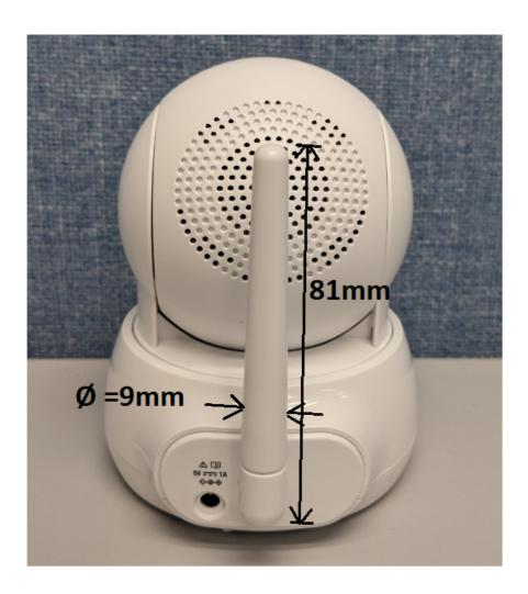
Figure 1 Physical dimension (mm)
