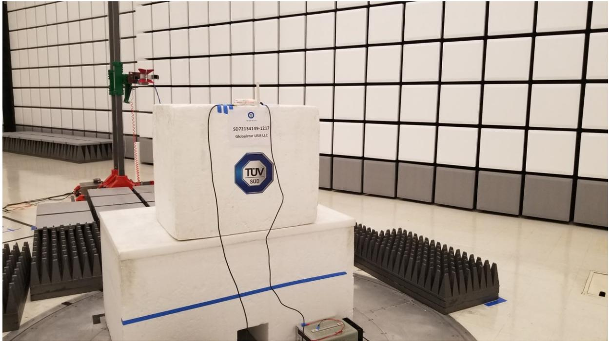
**Radiated Emissions Test Setup (above 1GHz)**
