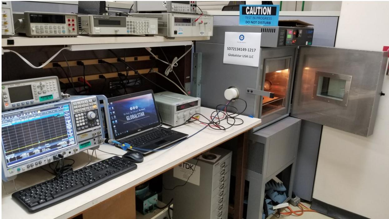
**Frequency Stability/Voltage Variation Test Setup**
