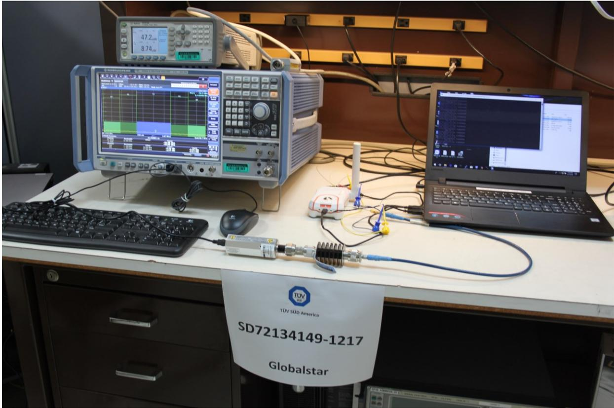
**Conducted Antenna Port Test Setup (WLAN)**
