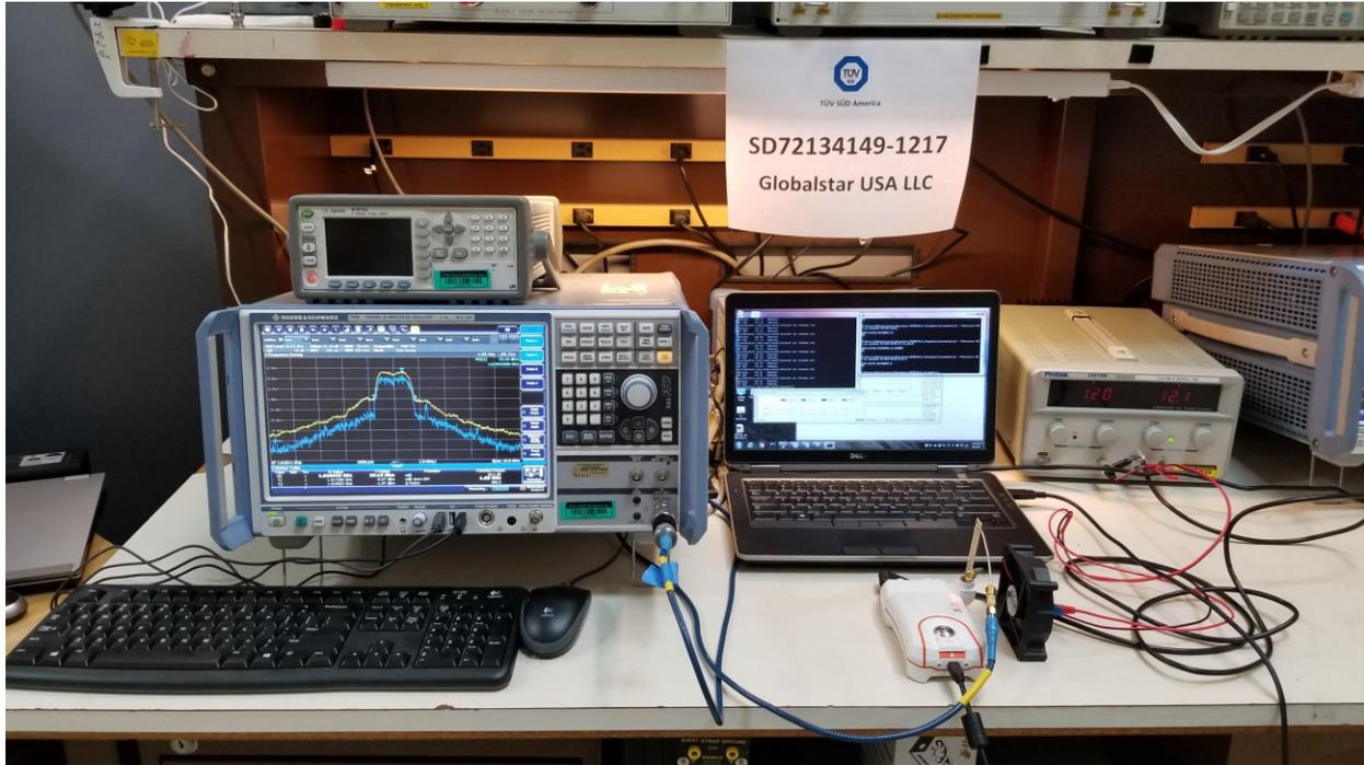
**Conducted Antenna Port Test Setup (Satellite)**
