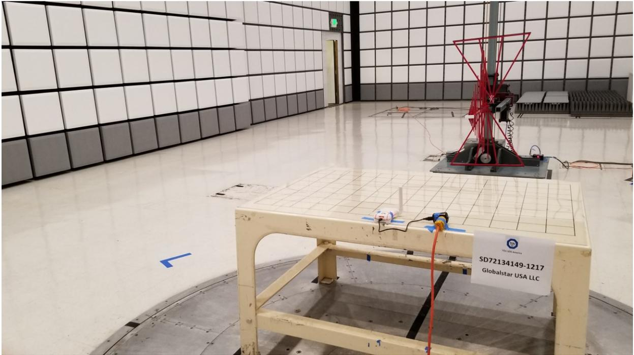
**Radiated Emissions Test Setup (below 30MHz)**
