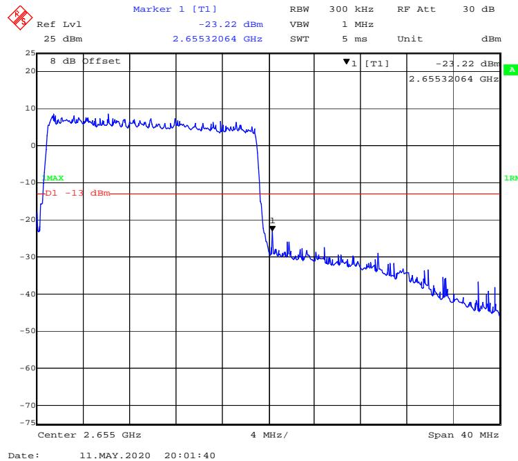
**16-QAM (5.0 MHz, FULL RB) - Left Band Edge**
