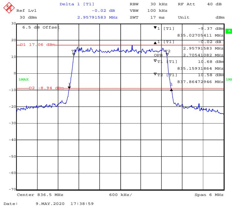
**16-QAM (5.0 MHz) - 99% Occupied & 26 dB Emissions Bandwidth, Middle channel**
