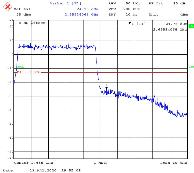
**16-QAM (10.0 MHz, FULL RB) - Left Band Edge**
