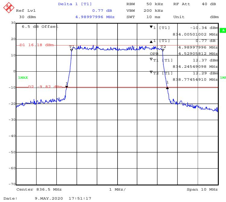
**16-QAM (10.0 MHz) - 99% Occupied & 26 dB Emissions Bandwidth, Middle channel**
