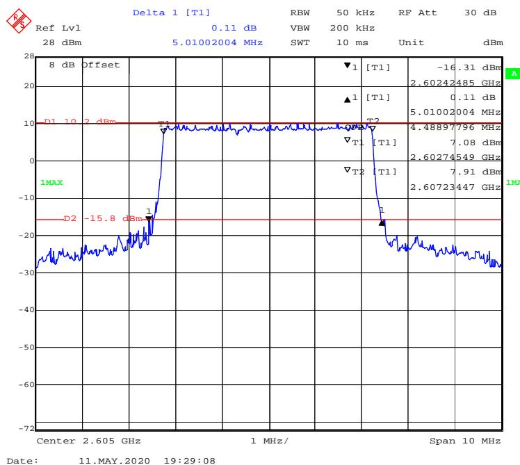
**QPSK (10.0 MHz) - 99% Occupied & 26 dB Emissions Bandwidth, Middle channel**
