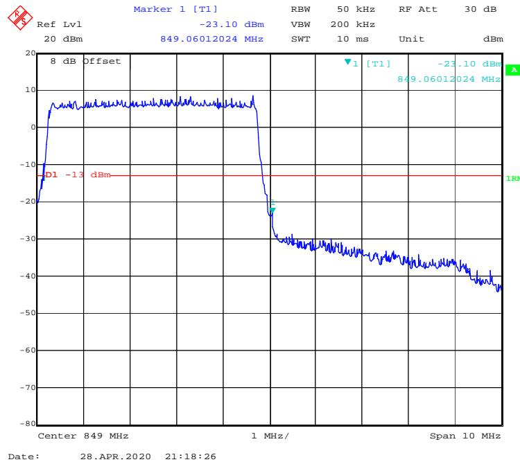
**QPSK (10.0 MHz, FULL RB) - Left Band Edge**
