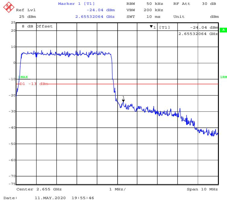
**QPSK (10.0 MHz, FULL RB) - Left Band Edge**
