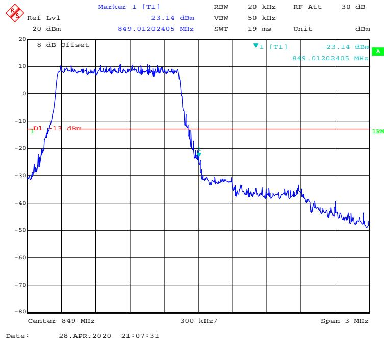
**16-QAM (3.0 MHz, FULL RB) - Left Band Edge**
