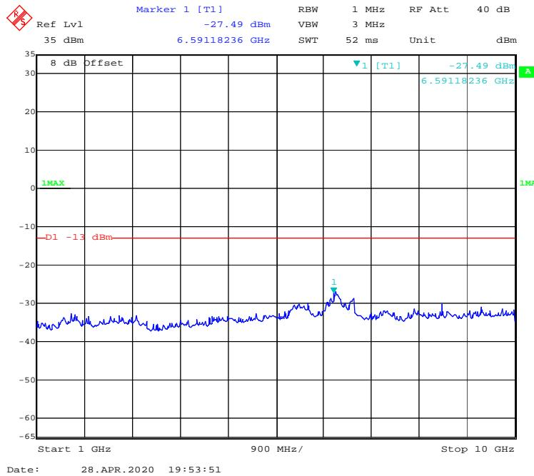
**30 MHz – 1GHz(EGPRS Mode)**
