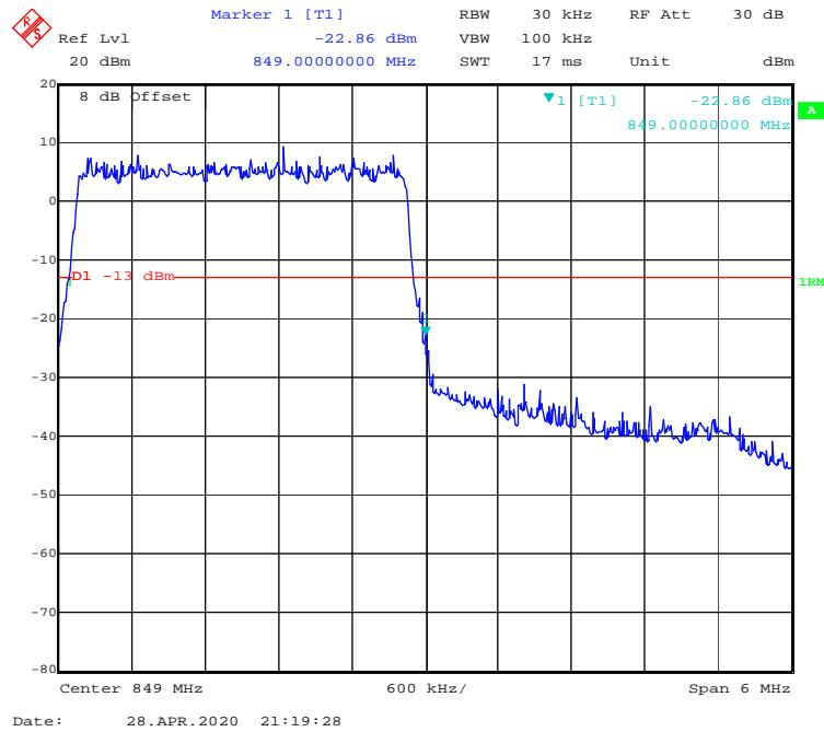
**16-QAM (5.0 MHz, FULL RB) - Left Band Edge**
