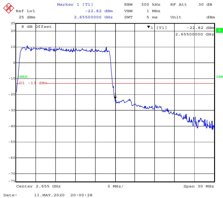
**16-QAM (20.0 MHz, FULL RB) - Left Band Edge**
