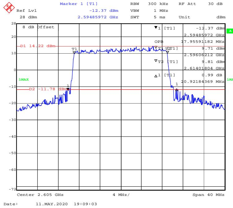
**16-QAM (5.0 MHz) - 99% Occupied & 26 dB Emissions Bandwidth, Middle channel**
