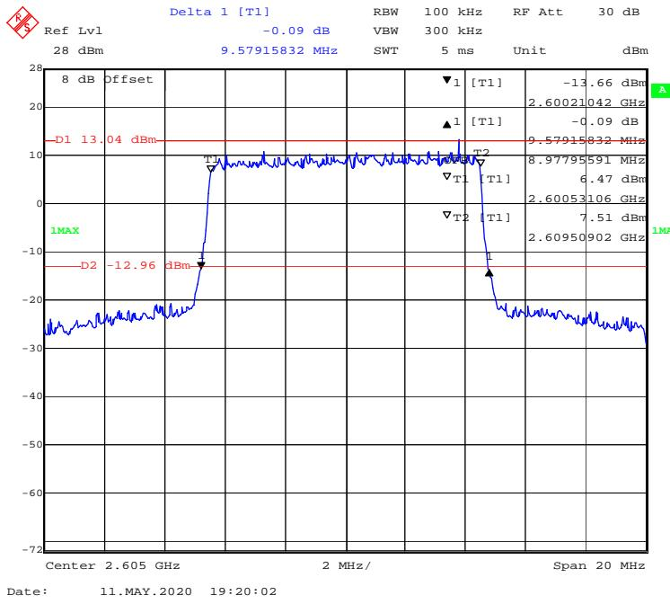
**16-QAM (15.0 MHz) - 99% Occupied & 26 dB Emissions Bandwidth, Middle channel**
