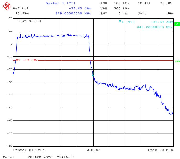
**16-QAM (1.4 MHz, FULL RB) - Left Band Edge**
