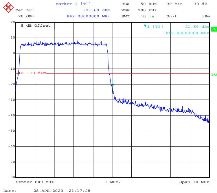
**16-QAM (10.0 MHz, FULL RB) - Left Band Edge**
