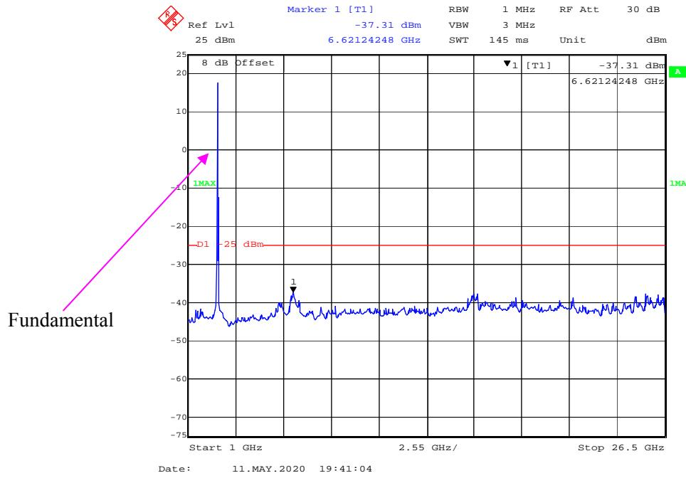
**FCC § 2.1053; § 22.917 (a); §27.53 (m) - SPURIOUS RADIATED EMISSIONS****Applicable Standards**
