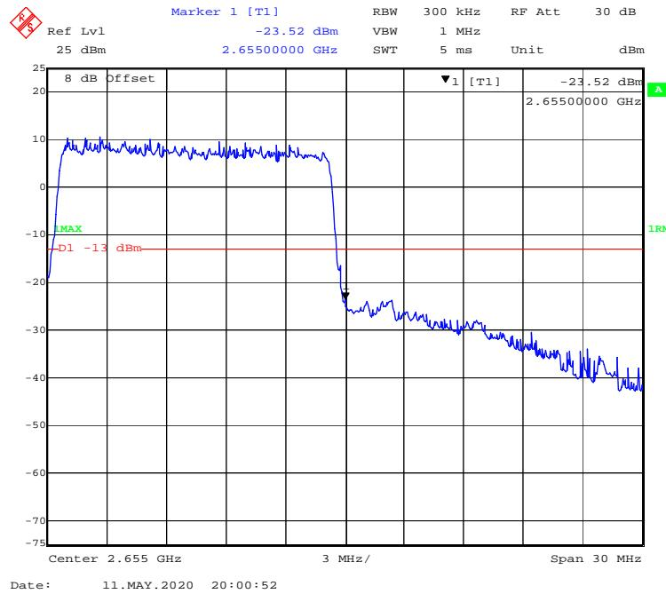
**QPSK (20.0 MHz, FULL RB) - Left Band Edge**
