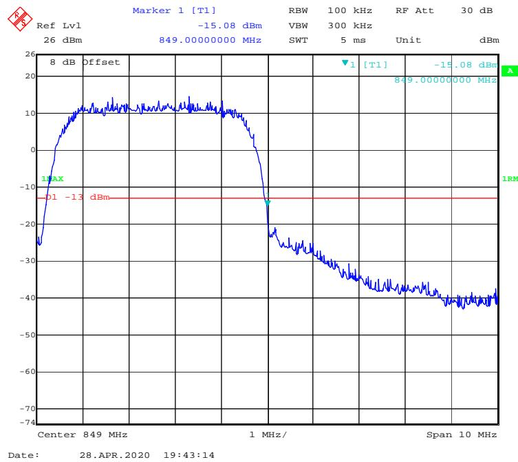
**LTE Band 5:****QPSK (1.4 MHz, FULL RB) - Left Band Edge**
