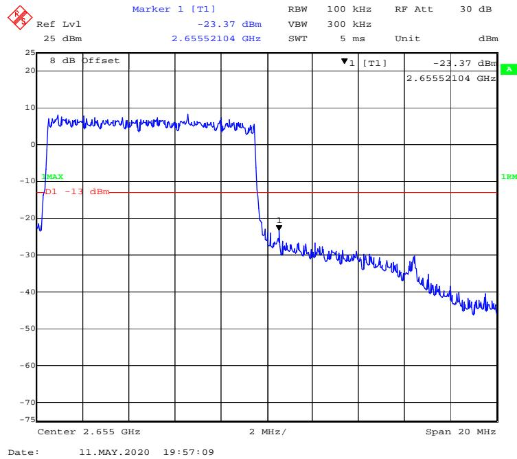
**QPSK (15.0 MHz, FULL RB) - Left Band Edge**
