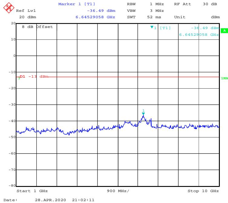
**30 MHz - 1 GHz (16QAM, 3.0 MHz, Middle Channel)**
