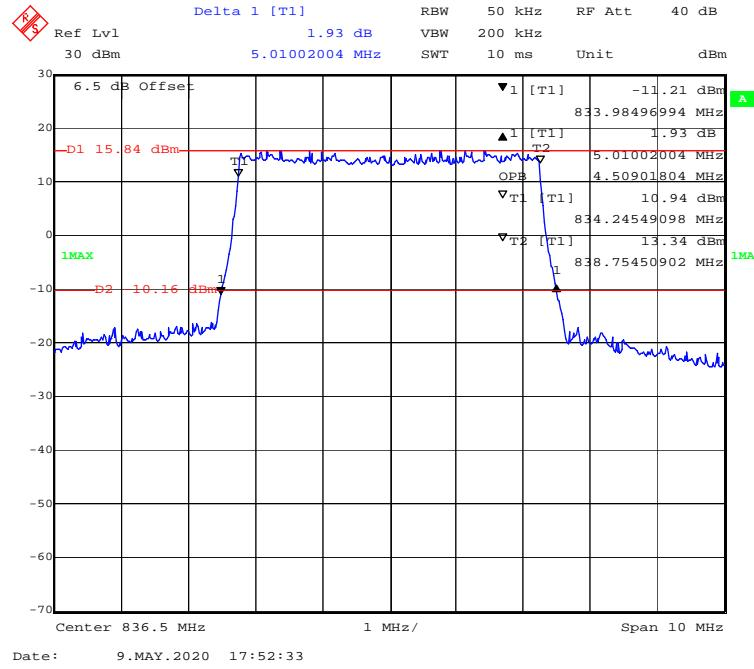
**QPSK (10.0 MHz) - 99% Occupied & 26 dB Emissions Bandwidth, Middle channel**
