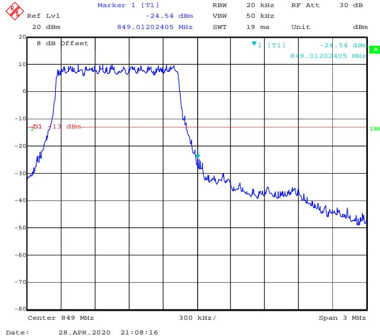
**QPSK (3.0 MHz, FULL RB) - Left Band Edge**
