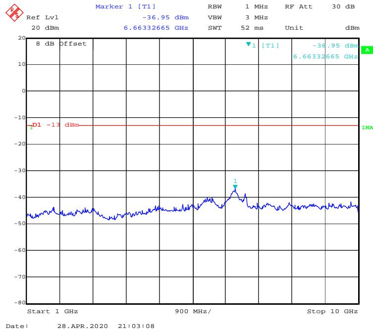
**30 MHz - 1 GHz (16QAM, 10.0 MHz, Middle Channel)**
