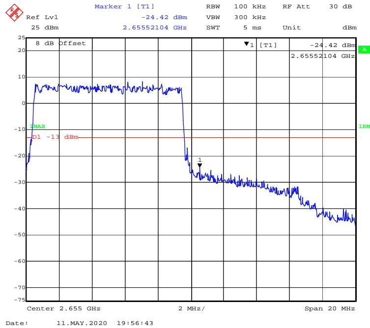
**16-QAM (15.0 MHz, FULL RB) - Left Band Edge**
