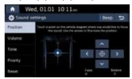
2. Adjust the sound position. Or press  $[\Lambda]/[V]/[<]/[>]$  to control the sound position.
