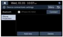
2. Press the [Add New] button to add the device to be connected or select a paired device and press the [Connect] button to connect.
