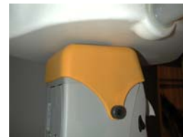
Figure 14.13 Body SAR Test Setup -- w/o Holster --
