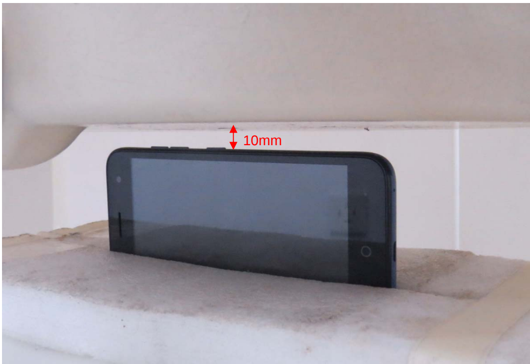
Picture 8: Right Side, the distance from handset to the bottom of the Phantom is 10mm
