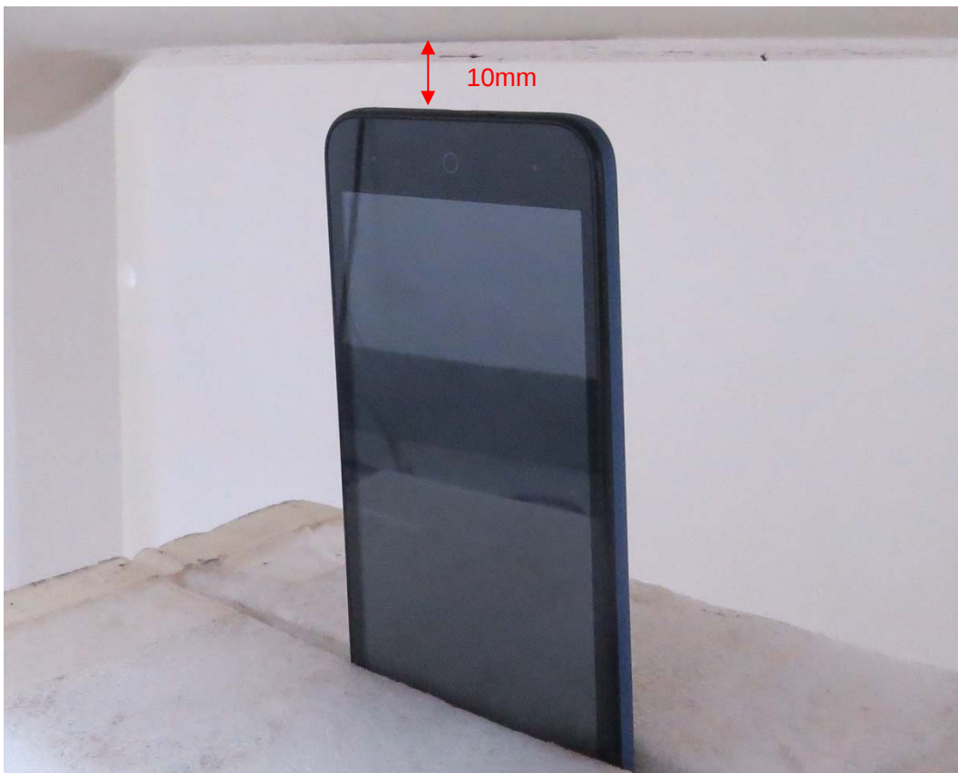
Picture 10: Bottom Side, the distance from handset to the bottom of the Phantom is 10mm
