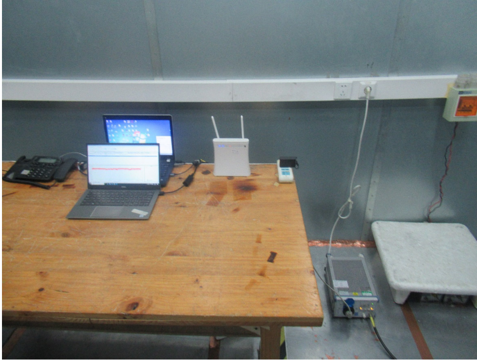
Picture 2: Conducted Emissions Test Setup
