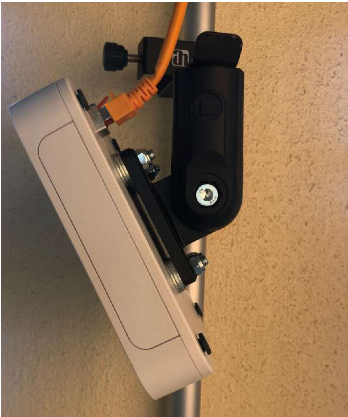
Figure 4: Anchor with tilt adjusted
