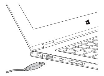
The first time you plug a USB device into a particular USB port on your computer, Windows automatically installs a driver for that device. After the driver has been installed, you can disconnect and reconnect the device without performing any additional steps.
