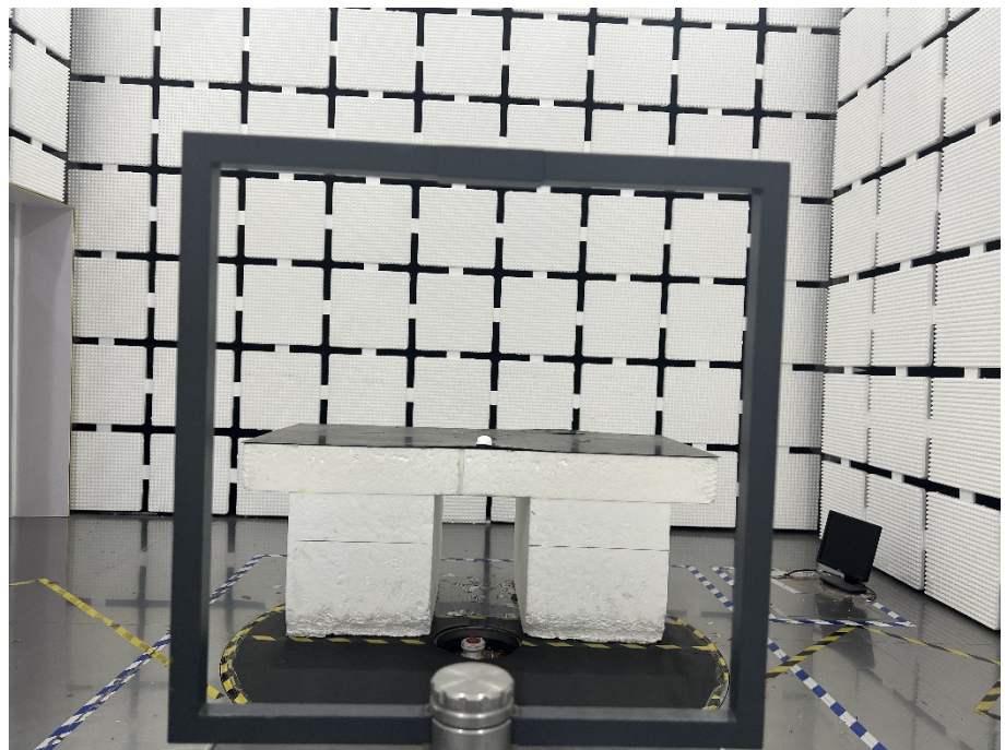
Radiation Emission Test Setup (Below 30MHz)
