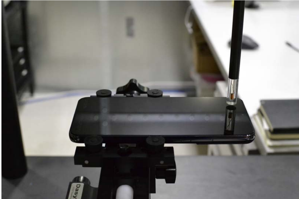
Figure 17-1 Test Setup for Wireless Device
