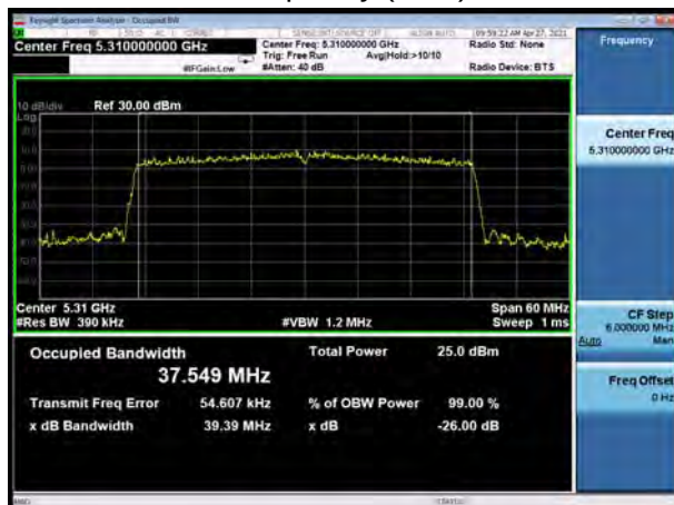
U-NII-2A, 802.11ax HE80 Carrier frequency (MHz): 5290
