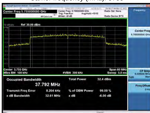
U-NII-3, 802.11ax HE40 Carrier frequency (MHz): 5755
