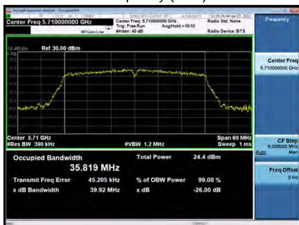
U-NII-2C, 802.11n HT40 Carrier frequency (MHz): 5710
