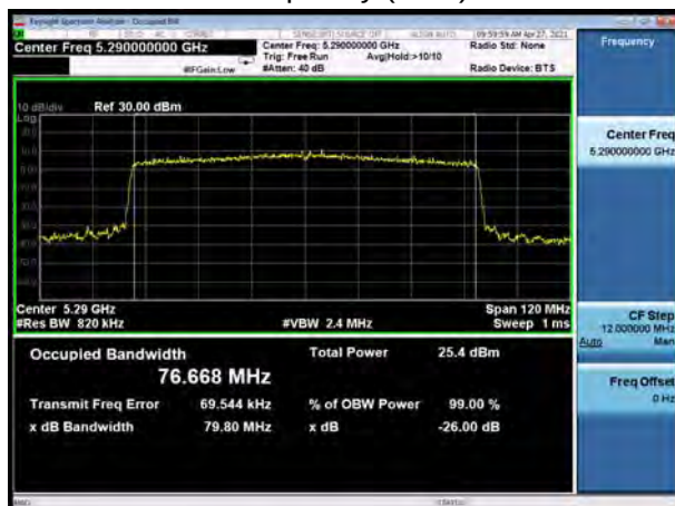
U-NII-2A, 802.11ax HE80 Carrier frequency (MHz): 5290
