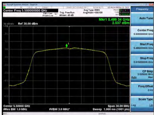
U-NII-2C, 802.11ac VHT20, Channel No.: 120
