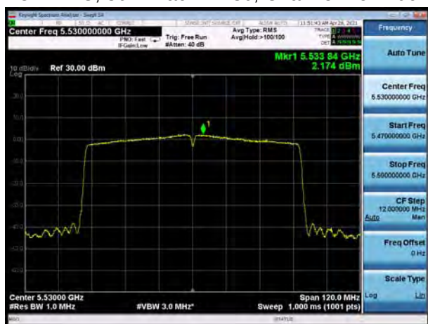
U-NII-2C, 802.11ac VHT80, Channel No.: 122
