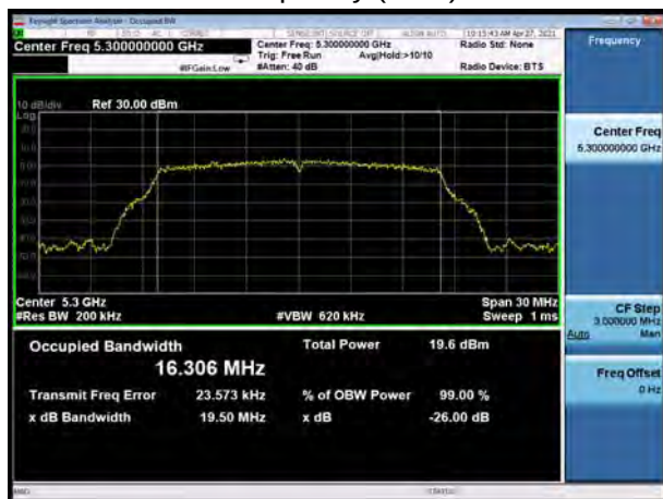
U-NII-2A, 802.11a Carrier frequency (MHz): 5300
