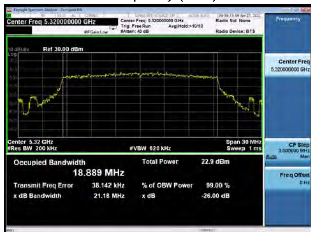
U-NII-2A, 802.11ax HE20 Carrier frequency (MHz): 5320
