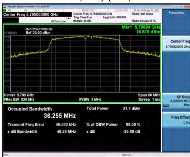
U-NII-3, 802.11n HT40 Carrier frequency (MHz): 5795
