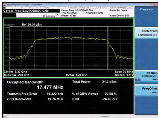
U-NII-2A, 802.11n HT20 Carrier frequency (MHz):5320
