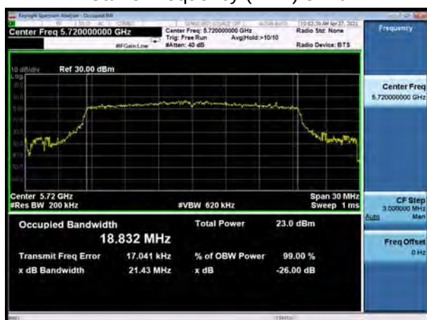
U-NII-2C, 802.11ax HE80 Carrier frequency (MHz): 5530
