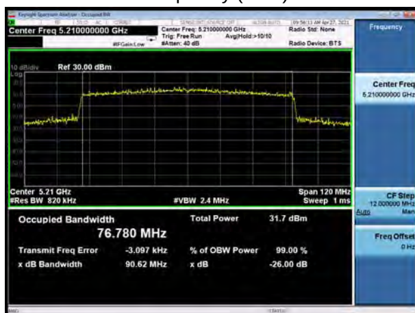
U-NII-1, 802.11ax HE80 Carrier frequency (MHz): 5210
