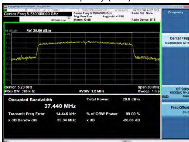
U-NII-1, 802.11ax HE40 Carrier frequency (MHz): 5230
