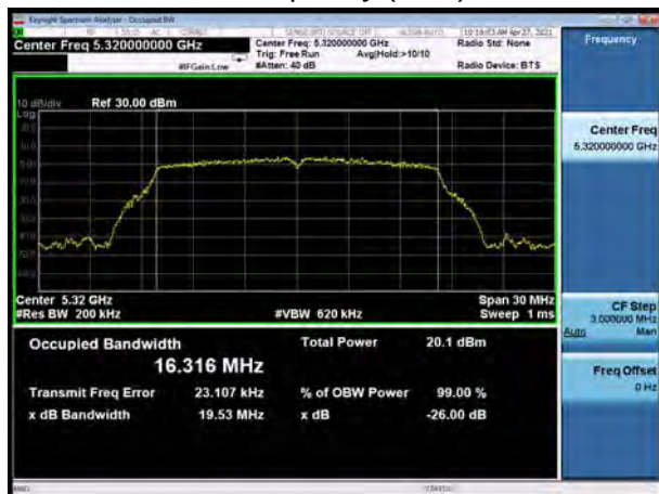
U-NII-2A, 802.11a Carrier frequency (MHz):5320
