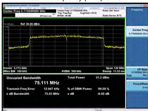
U-NII-3, 802.11ax HE40 Carrier frequency (MHz): 5755
