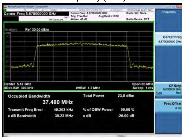
U-NII-2C, 802.11ax HE40 Carrier frequency (MHz): 5710
