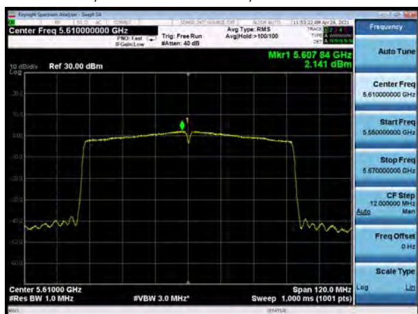
U-NII-2C, 802.11ac VHT80, Channel No.: 122
