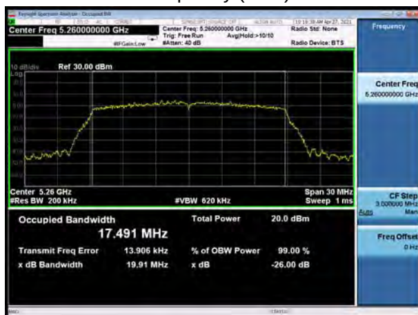
U-NII-2A, 802.11n HT20 Carrier frequency (MHz): 5300
