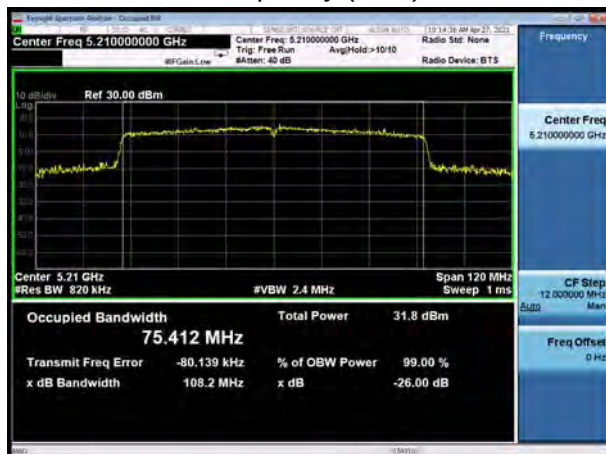
U-NII-1, 802.11ax HE40 Carrier frequency (MHz): 5190
