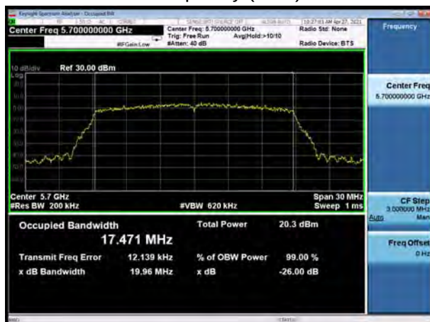
U-NII-2C, 802.11n HT20 Carrier frequency (MHz): 5720
