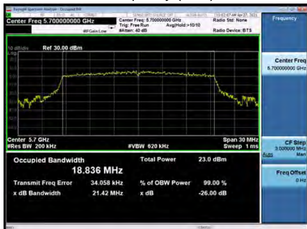
U-NII-2C, 802.11ax HE20 Carrier frequency (MHz): 5720
