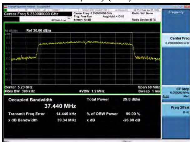
U-NII-1, 802.11ax HE40 Carrier frequency (MHz): 5230
