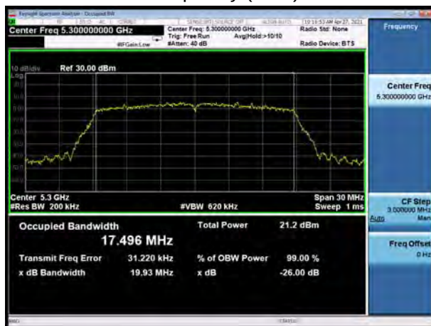
U-NII-2A, 802.11n HT20 Carrier frequency (MHz): 5300
