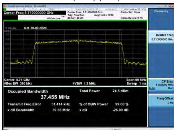
U-NII-2C, 802.11ax HE40 Carrier frequency (MHz): 5710
