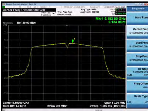
U-NII-1, 802.11ac VHT40, Channel No.: 38
