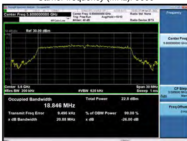
U-NII-2C, 802.11ax HE20 Carrier frequency (MHz): 5600
