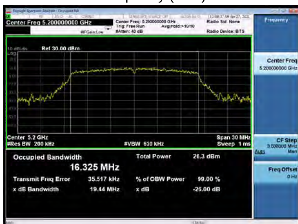
U-NII-1, 802.11a Carrier frequency (MHz): 5240
