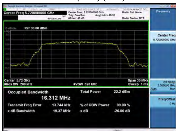
U-NII-2C, 802.11a Carrier frequency (MHz): 5720
