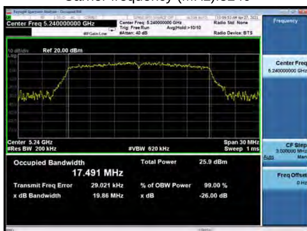
U-NII-1, 802.11n HT20 Carrier frequency (MHz): 5240
