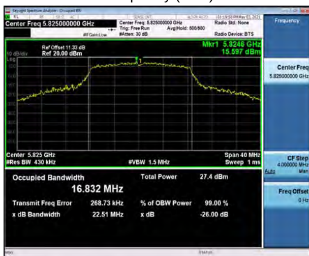
U-NII-3, 802.11n HT40 Carrier frequency (MHz): 5755
