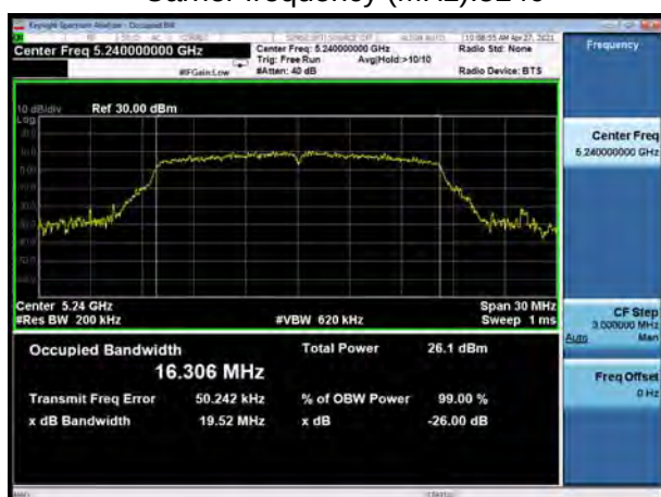
U-NII-1, 802.11a Carrier frequency (MHz): 5240
