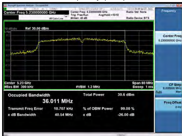
U-NII-1, 802.11ax HE20 Carrier frequency (MHz): 5180
