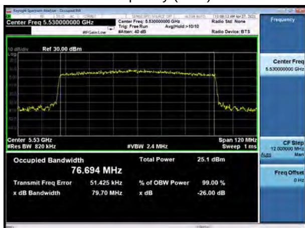
U-NII-2C, 802.11ax HE80 Carrier frequency (MHz): 5530
