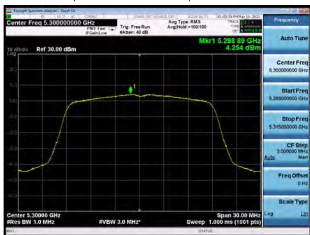
U-NII-2A, 802.11ac VHT20, Channel No.: 60
