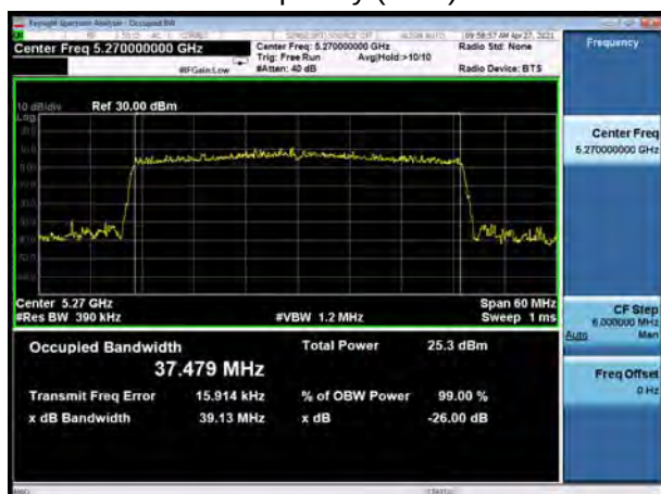
U-NII-2A, 802.11ax HE40 Carrier frequency (MHz): 5270
