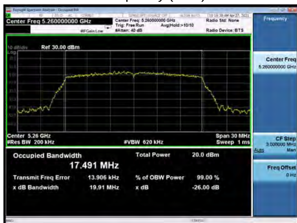
U-NII-2A, 802.11n HT20 Carrier frequency (MHz): 5300
