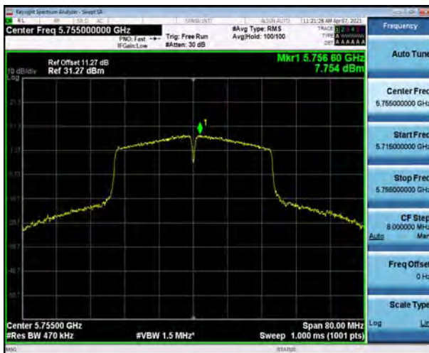
U-NII-3, 802.11ac VHT40, Channel No.: 159
