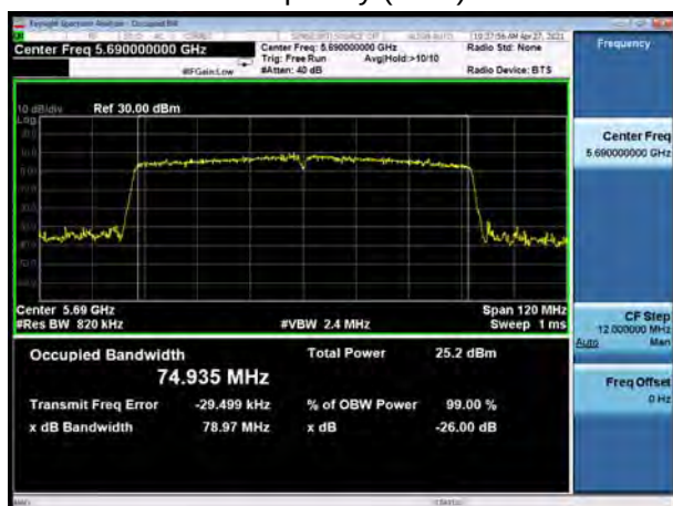
U-NII-2C, 802.11ax HE20 Carrier frequency (MHz): 5500
