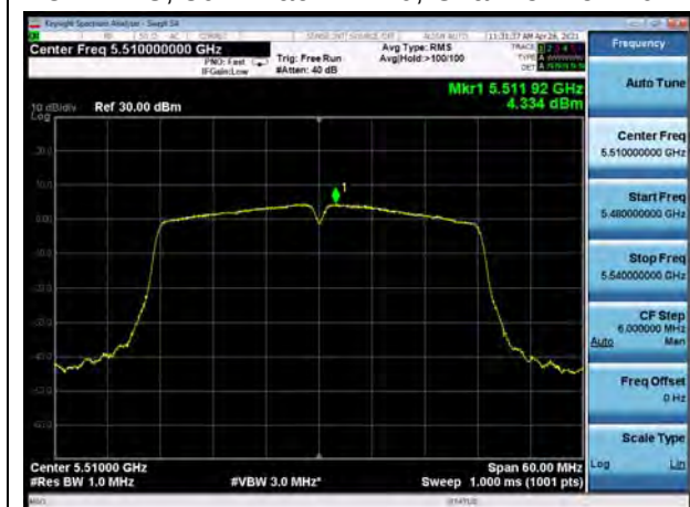
U-NII-2C, 802.11ac VHT40, Channel No.: 118
