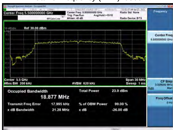
U-NII-2C, 802.11ax HE20 Carrier frequency (MHz): 5600
