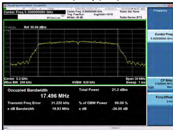
U-NII-2A, 802.11n HT20 Carrier frequency (MHz): 5300
