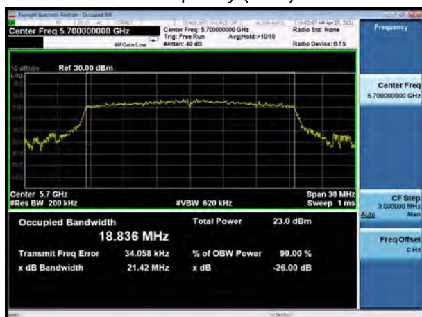
U-NII-2C, 802.11ax HE20 Carrier frequency (MHz): 5720
