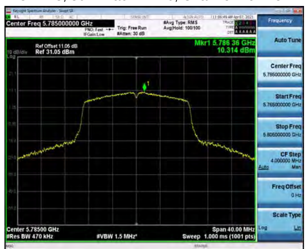
U-NII-3, 802.11ac VHT20, Channel No.: 157
