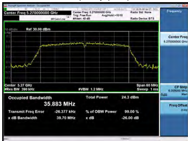
U-NII-2A, 802.11n HT40 Carrier frequency (MHz): 5310
