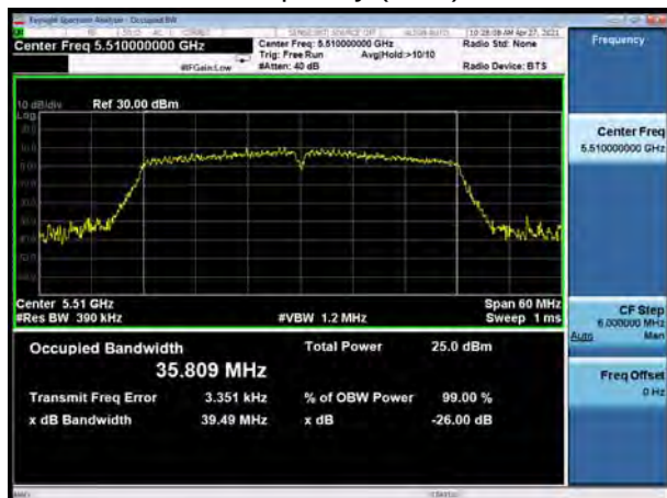
U-NII-2C, 802.11n HT40 Carrier frequency (MHz): 5590
