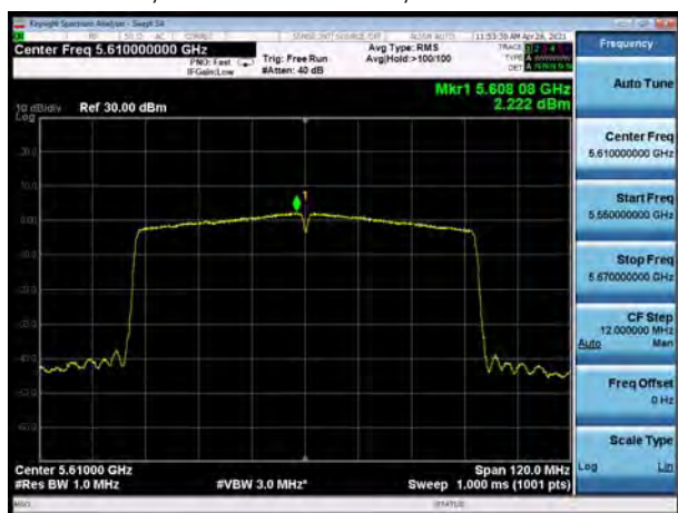
U-NII-2C, 802.11ac VHT80, Channel No.: 122
