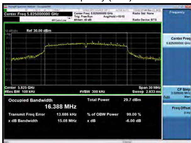
U-NII-3, 802.11n HT40 Carrier frequency (MHz): 5755
