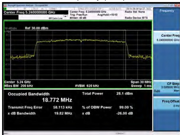
U-NII-1, 802.11ax HE20 Carrier frequency (MHz):5240
