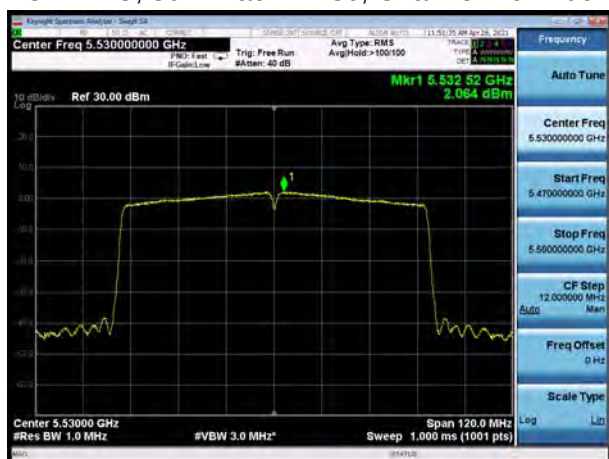
U-NII-2C, 802.11ac VHT80, Channel No.: 122
