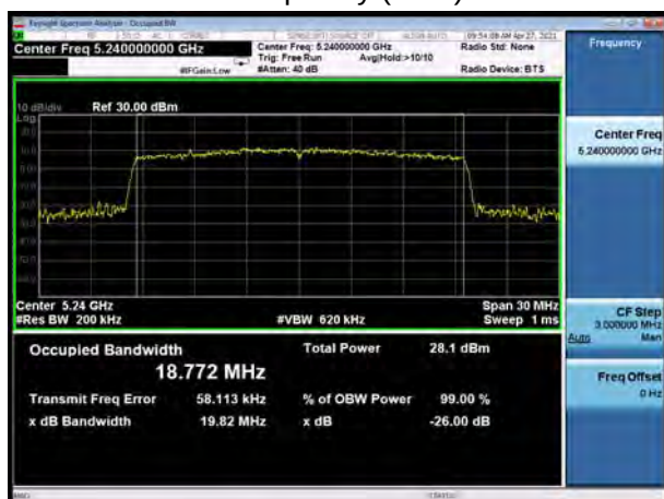
U-NII-1, 802.11ax HE20 Carrier frequency (MHz):5240
