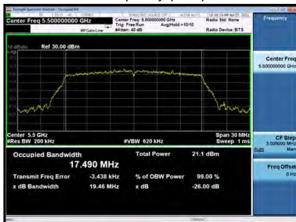
U-NII-2C, 802.11n HT20 Carrier frequency (MHz): 5500
