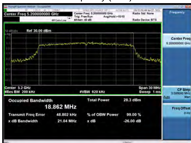
U-NII-1, 802.11ax HE20 Carrier frequency (MHz): 5200
