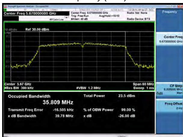
U-NII-2C, 802.11n HT40 Carrier frequency (MHz): 5670
