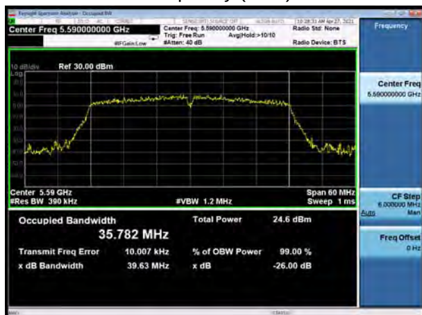
U-NII-2C, 802.11n HT40 Carrier frequency (MHz): 5670
