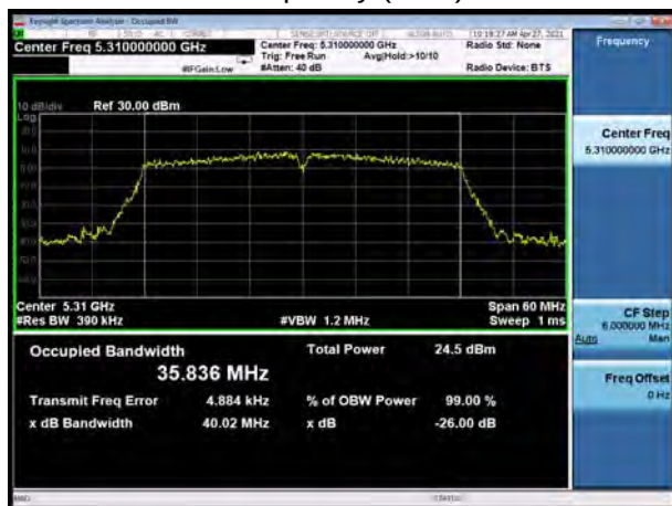
U-NII-2A, 802.11n HT40 Carrier frequency (MHz): 5310
