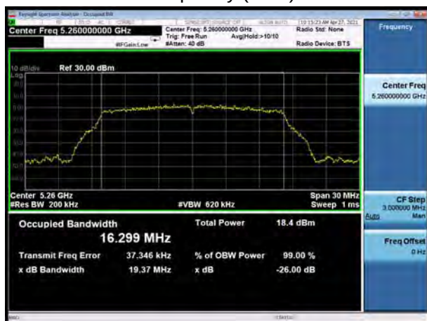
U-NII-2A, 802.11a Carrier frequency (MHz): 5300
