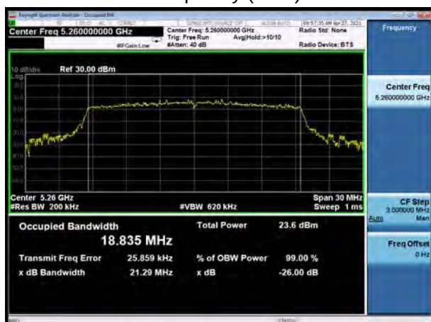
U-NII-2A, 802.11ax HE20 Carrier frequency (MHz): 5260
