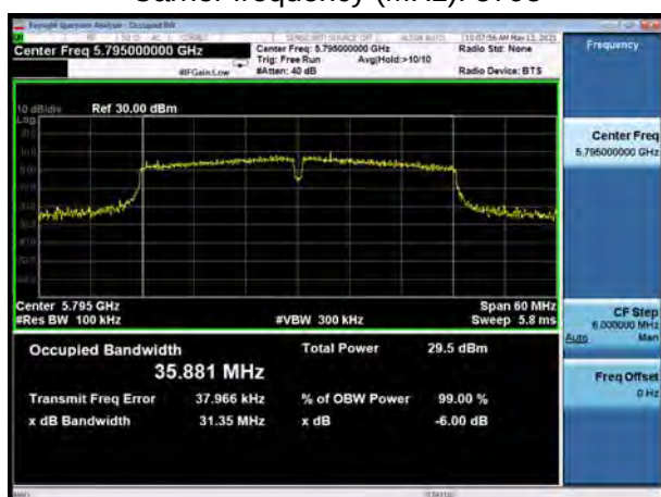
U-NII-3, 802.11n HT40 Carrier frequency (MHz): 5795
