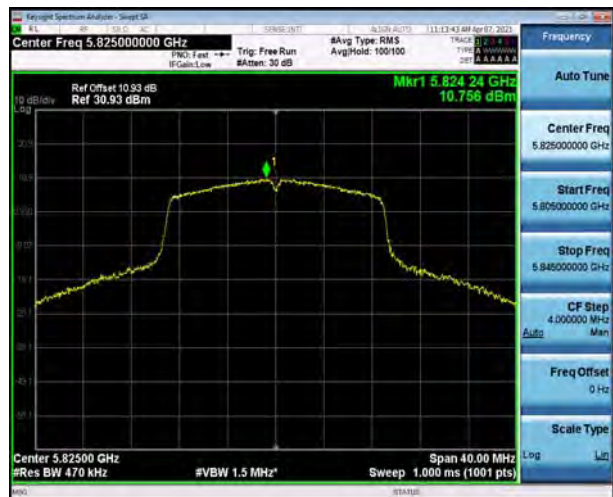
U-NII-3, 802.11ac VHT80, Channel No.: 155
