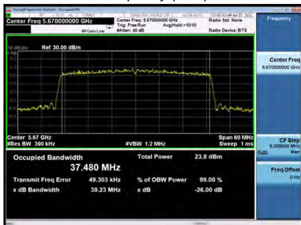
U-NII-2C, 802.11ax HE40 Carrier frequency (MHz): 5710
