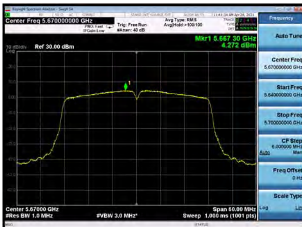
U-NII-2C, 802.11ac VHT40, Channel No.: 142
