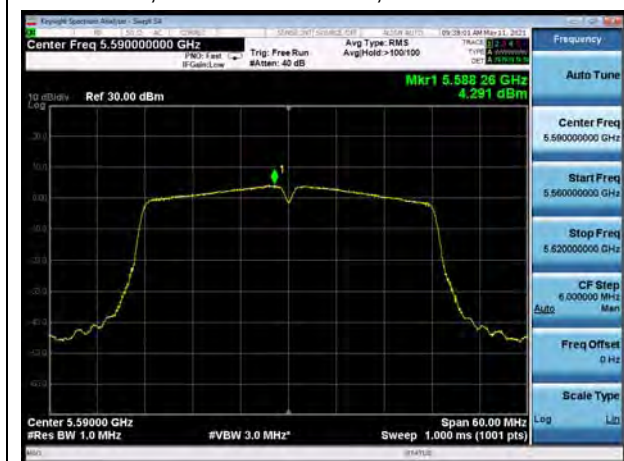
U-NII-2C, 802.11ac VHT40, Channel No.: 118
