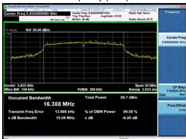
U-NII-3, 802.11n HT40 Carrier frequency (MHz): 5755
