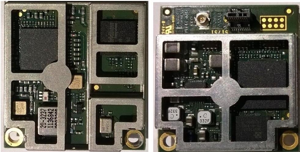
Figure 1 - Iridium 9603N top and bottom side views with casing removed
