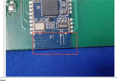
The antenna is PCB antenna.
