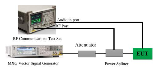
2. Apply a signal to the EUT antenna port at lowest, middle, highest channel frequencies of the operating band;
