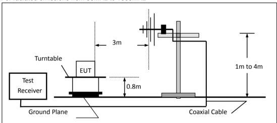
(c) For radiated emissions above 1000MHz
