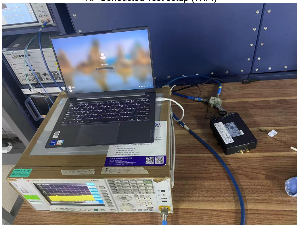
RF Conducted Test setup (LTE)
