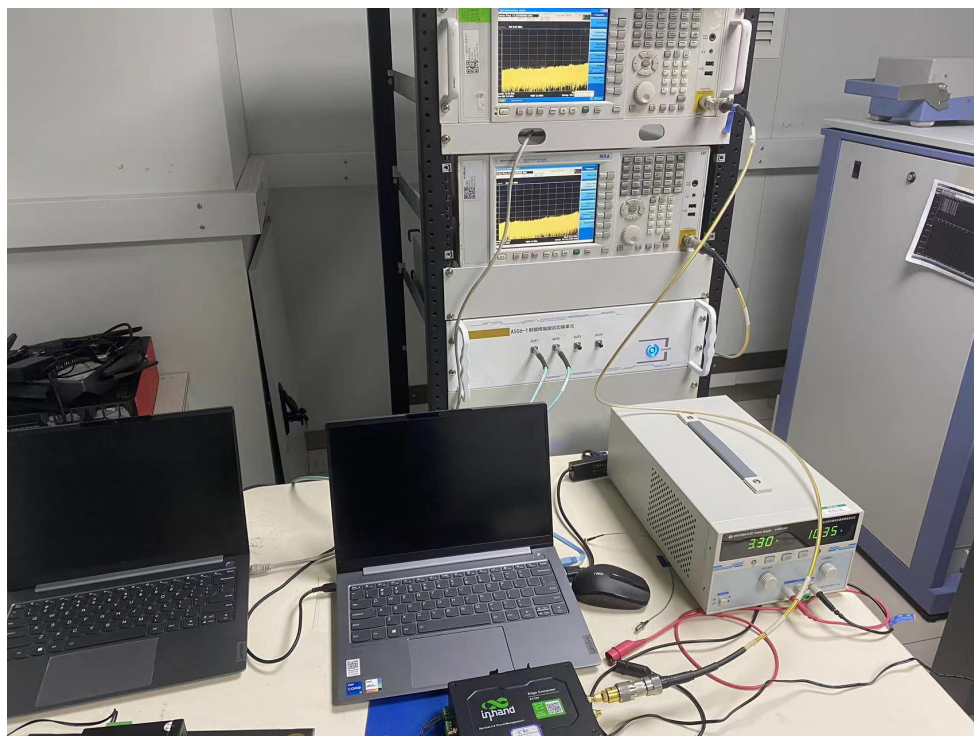
RF Conducted Test setup (WIFI)
