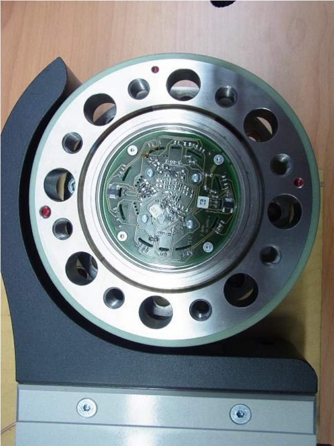
The rotor includes 4 PCB
