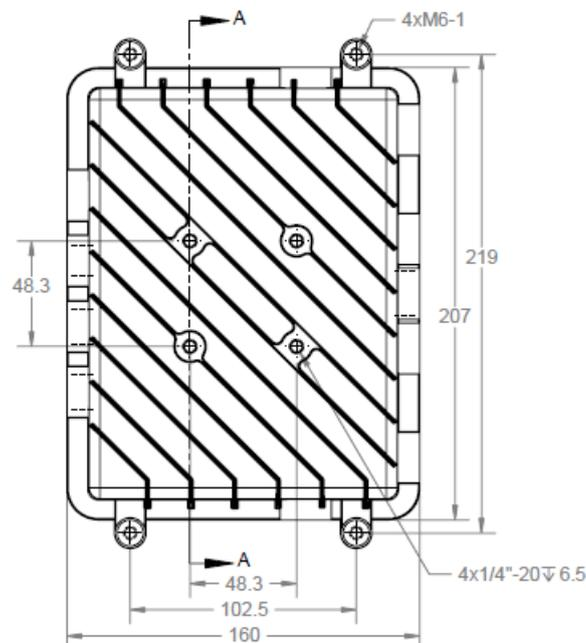
**FIGURE 8 - XBU ENCLOSURE MOUNTING HOLE**
