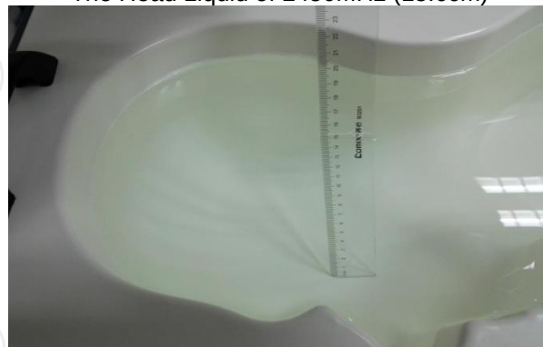
The Head Liquid of 1800MHz (15.2cm)
