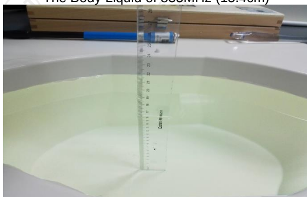
The Body Liquid of 1900MHz (16.4 cm)
