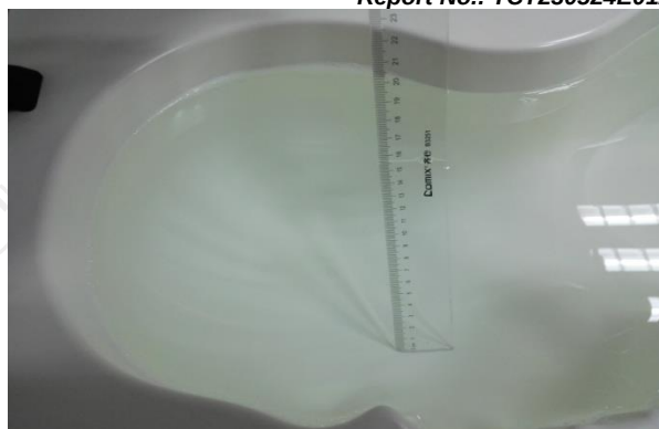
The Head Liquid of 2450MHz (15.6cm)
