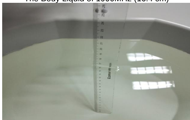
The Body Liquid of 5000-6000MHz (16.5cm)
