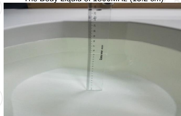
The Body Liquid of 2450MHz (15.3cm)
