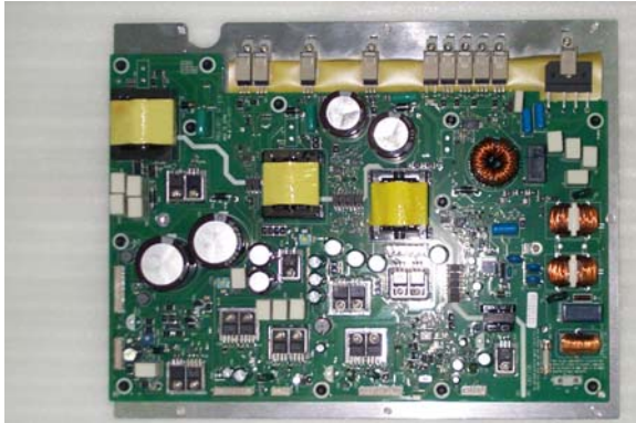
Original DSP-4280GM power board (Manufactured by SM TECH)
