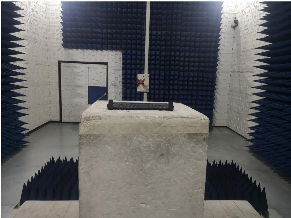
FCC RADIATED EMISSION TEST SETUP ABOVE 1GHZ
