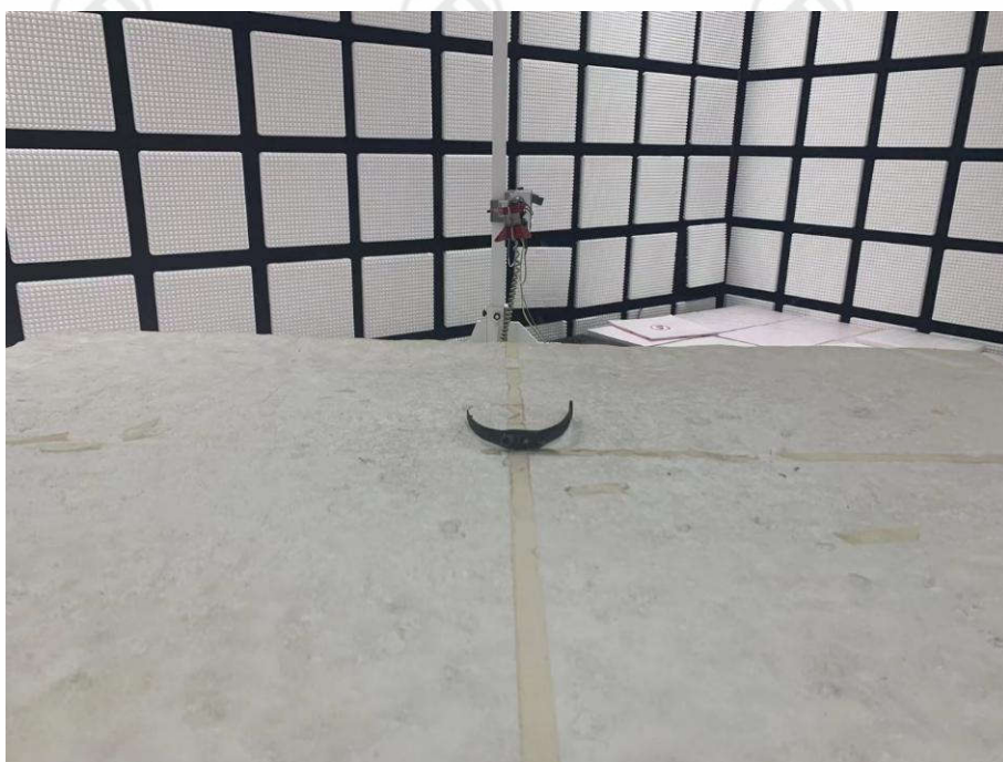
Radiated spurious emission Test Setup-2(Above 1GHz)
