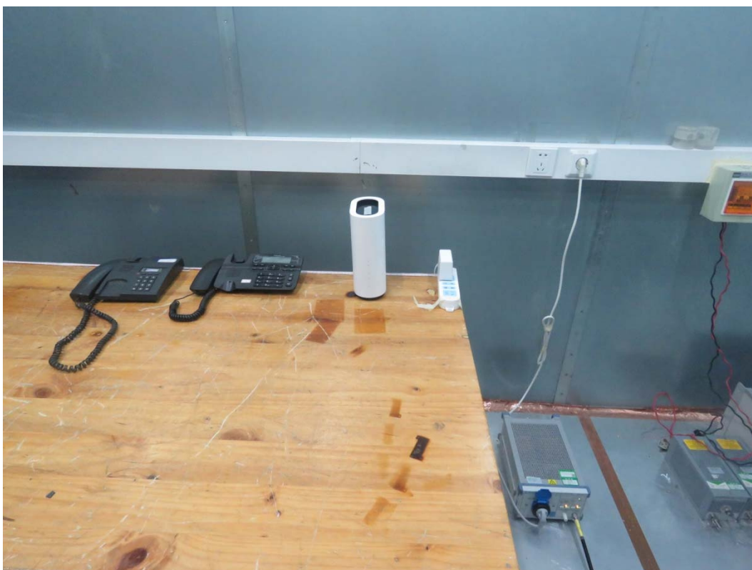
Picture 2: Conducted Emissions Test Setup
