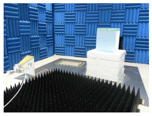
Radiated Emission for above 1GHz – FCC Part 24 Subpart E
