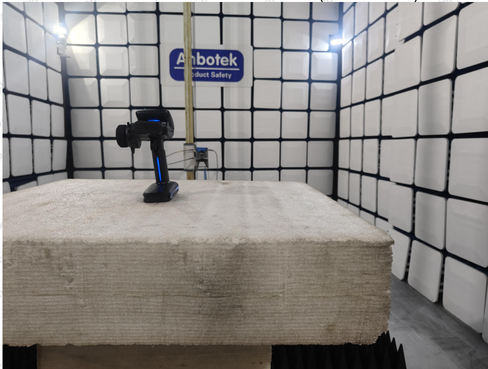
Photo of Radiation Emission Test (above 1GHz)
