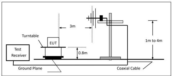
(c) For radiated emissions above 1000MHz
