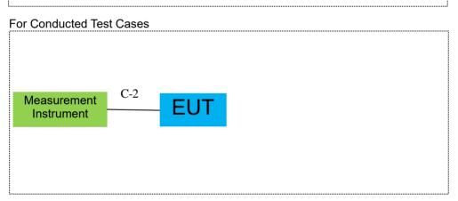
Note: 1. The temporary antenna connector is soldered on the PCB board in order to perform conducted tests and this temporary antenna connector is listed in the equipment list.
