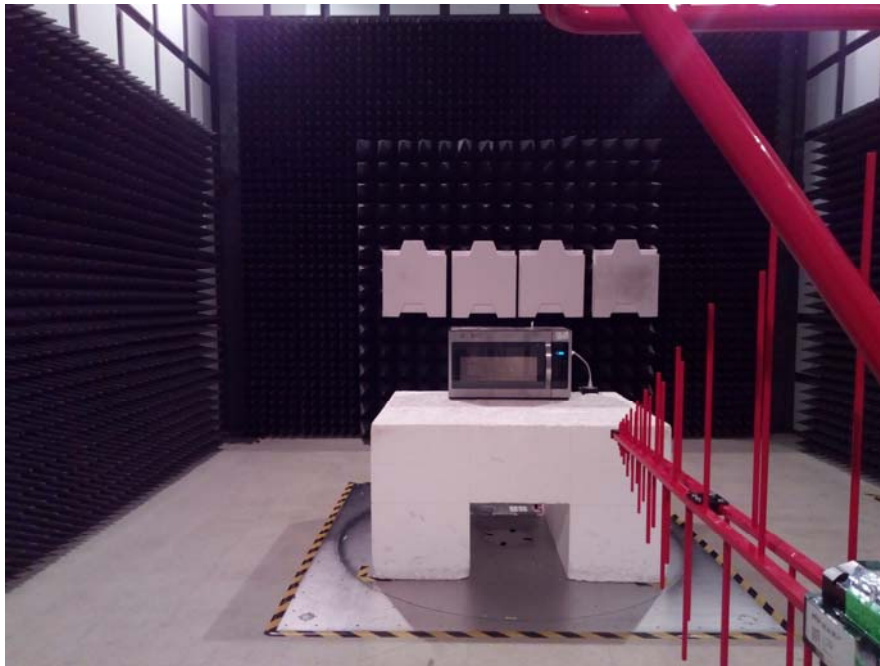
Radiated Emissions – Front View (30 MHz – 1 GHz)
