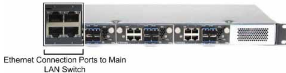
Figure 6-2. CEM LAN and Fiber Connection Ports
