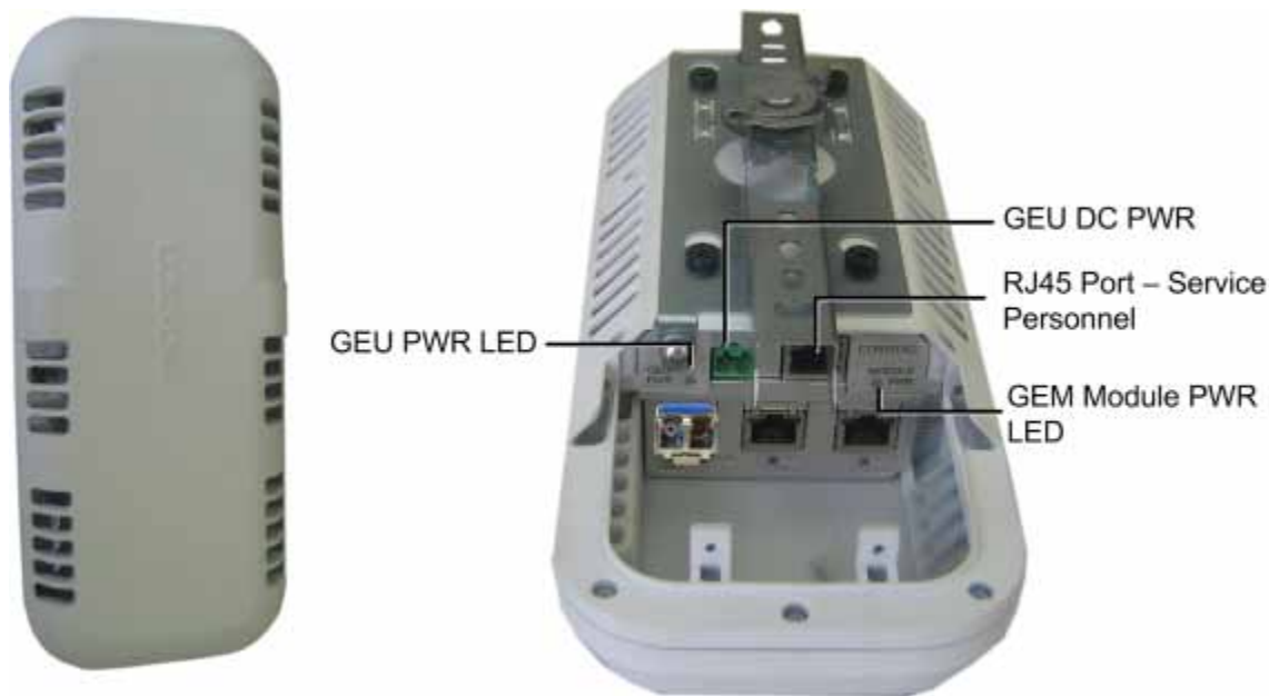
Figure 3-6. GEU Enclosure: Top (Left) and Open Underside (Right)
