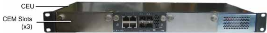
Figure 3-2. CEU Front Panel with Installed CEM Module
