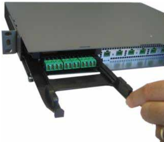
Figure 5-45. Edge Module Flush with Panel (Chassis Front)
