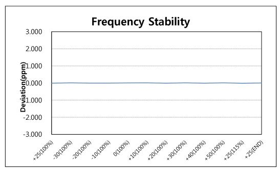
**Note.** Based on the results of the frequency stability test at the center channel the frequency deviation results measured are very small. as such it is determined that the channels at the band edge would remain inband when the maximum measured frequency deviation noted during the frequency stability tests is applied. therefore the device is determined to remain operating in band over the temperature and voltage range as tested.
