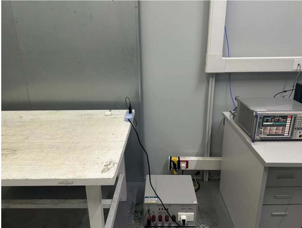
Photos of power line conducted emission test
