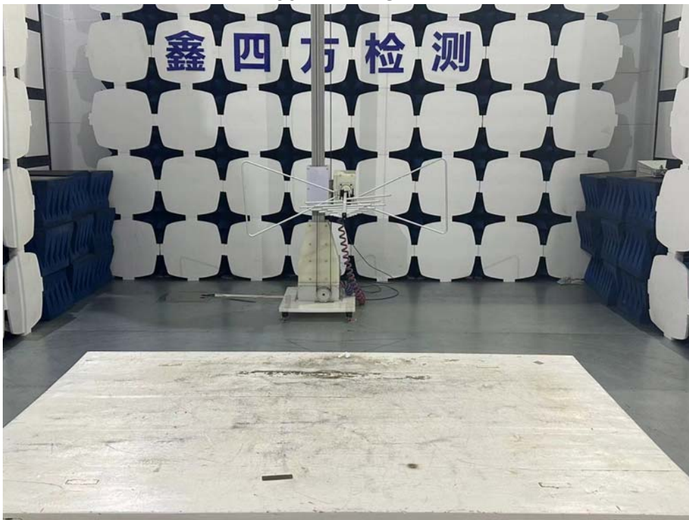
Photos of radiated emission test 30MHz – 1GHz
