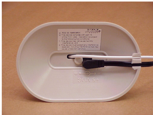
Figure 4 – Plugging the DC Power Connector into the Bottom Jack of the Max Ranger
