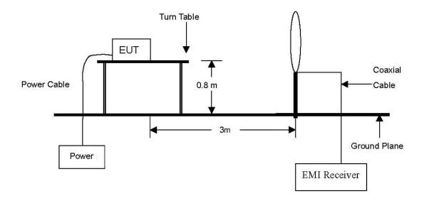
The diagram below shows the test setup that is utilized to make the measurements for emission from 30  $\,\mathrm{Mz}$  to 1  $\,\mathrm{GHz}$ .
