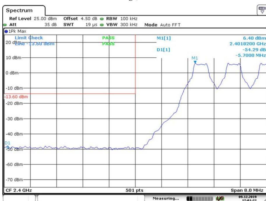
**Band Edge, Right Side**
