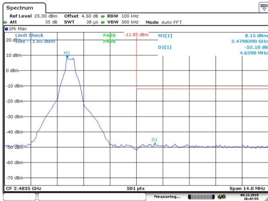
*EDR Mode ( $\pi/4$ -DQPSK):***Band Edge, Left Side**
