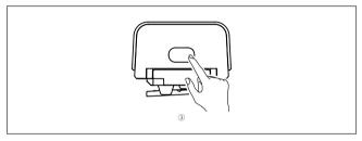
3. Press the power button for 3 seconds to turn on the lamp
