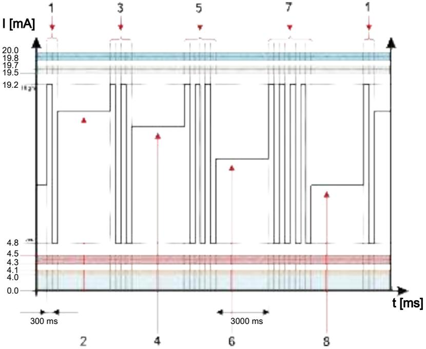
Fig. 37: Example: Analogue output signal NAS classes 2-5  $\mu\text{m}$  / 5-15  $\mu\text{m}$  / 15-25  $\mu\text{m}$  /  $\geq 25 \mu\text{m}$ , time-coded
