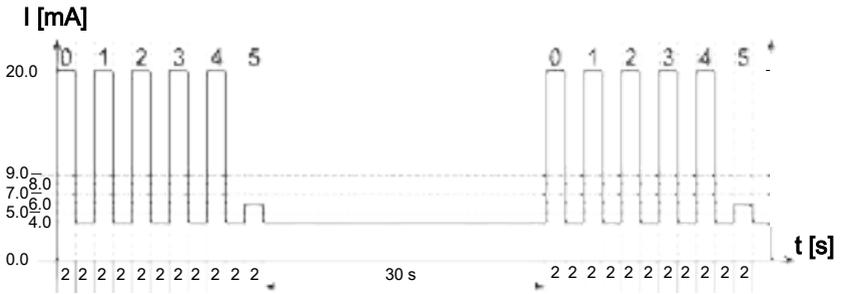
Fig. 35: Example: status of analogue signal 5
