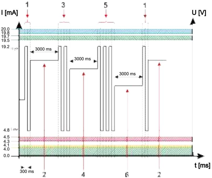
Fig. 32: Example: Analogue output signal ISO code, time-coded
