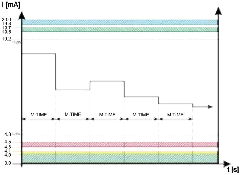
Fig. 20: Example: Analogue output signal class SAE A / SAE B / SAE C or SAE D
