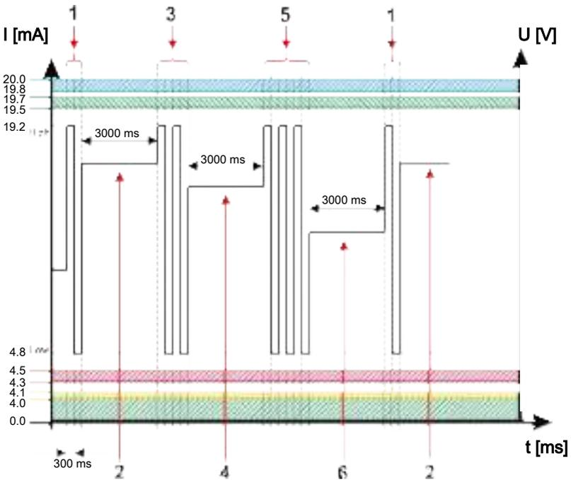
Fig. 26: Example: Analogue output signal ISO code, time-coded
