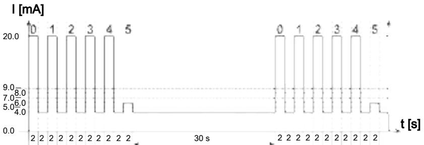
Fig. 23: Example: status of analogue signal 5
