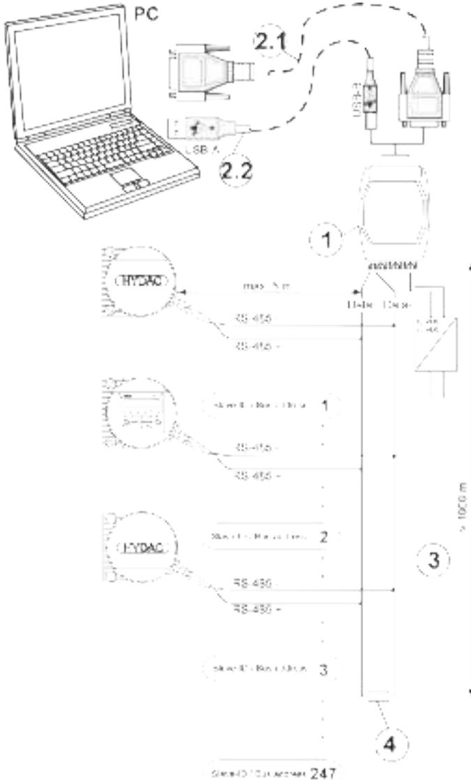
Fig. 18: Connecting / reading out ContaminationSensor via RS485
