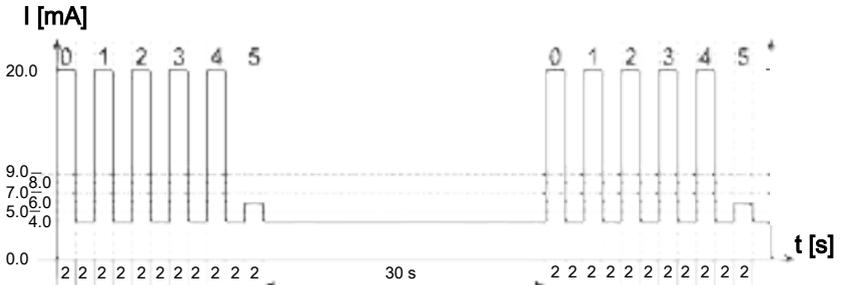
Fig. 43: Example: status of analogue signal 5
