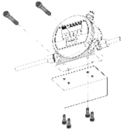
Fig. 8: Mounting on a wall or bracket
