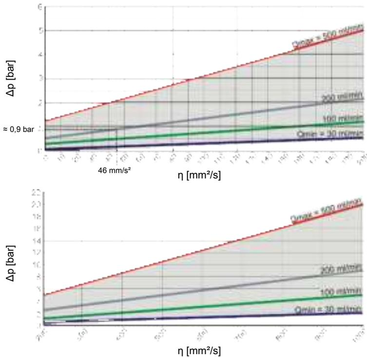
Fig. 12: Flow rate, differential pressure and viscosity characteristics
