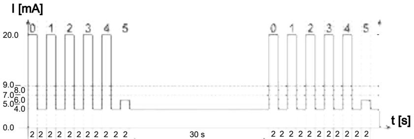
Fig. 41: Example: status of analogue signal 5
