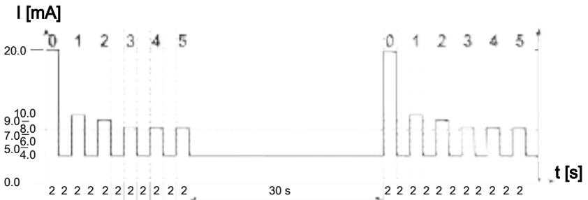
Fig. 44: Example: HDA-signal output – signal 1 to 4
