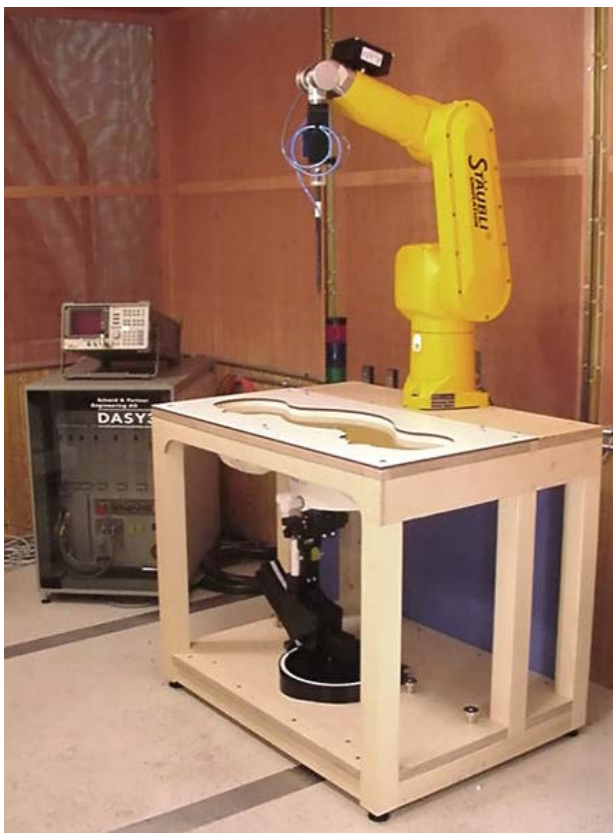
DASY3 SAR Measurement System with SAM Phantom
