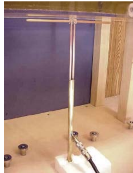
450MHz Dipole Validation Setup
