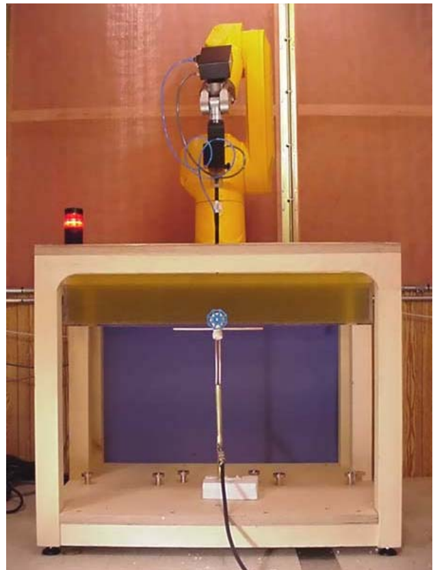
DASY3 SAR Measurement System with validation phantom
