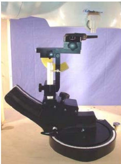
Face-held SAR Test Setup
