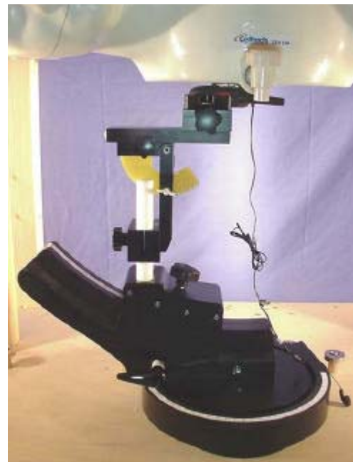
Body-worn SAR Test Setup
