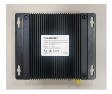
Label pasting position: On the back of the host, align it up and down in the center and paste it
