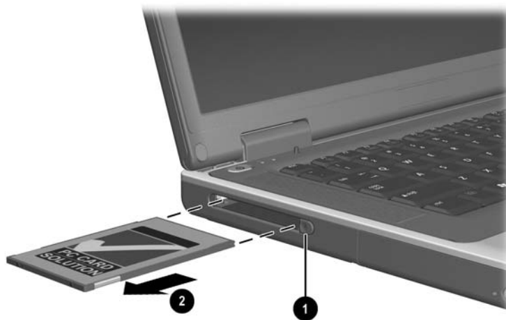
Removing a PC Card
