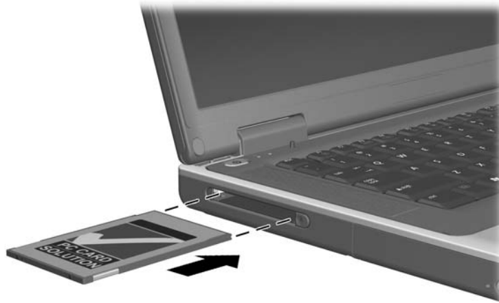
Inserting a PC Card
