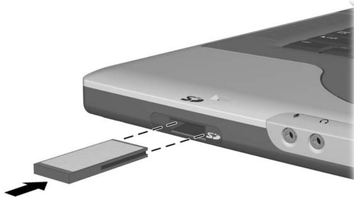
Inserting an SD Card or MMC
