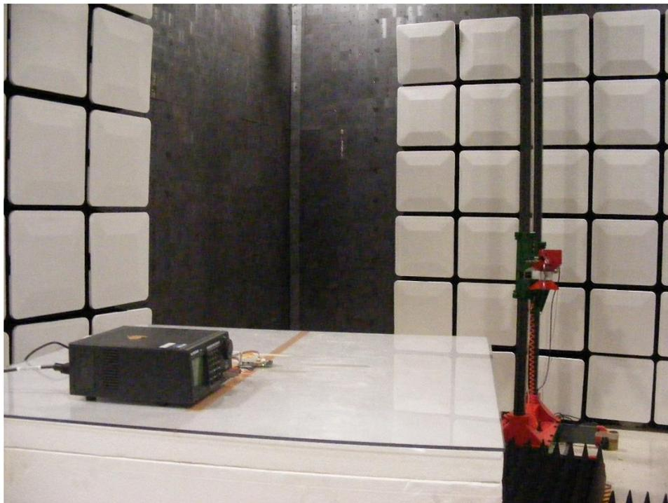
*Figure 8.1-8: Radiated emissions 1 GHz-18 GHz - Back*
