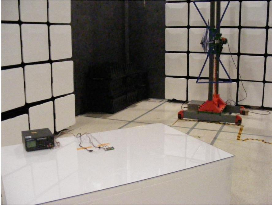
**Figure 8.1-5: Radiated emissions 30 MHz-1 GHz Front Picture**
