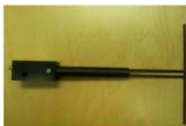
Figure 1 – MVG COMOSAR Validation Dipole
