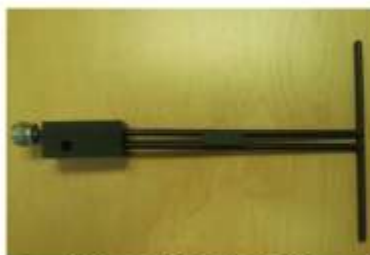
Figure 1 – MVG COMOSAR Validation Dipole
