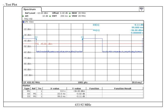
The average field strength may be found by measuring the peak pulse amplitude (in log equivalent units) and determining the duty cycle correction factor (in dB) associated with the pulse modulation as shown in Equation. (ANSI C63.10: 2020)
